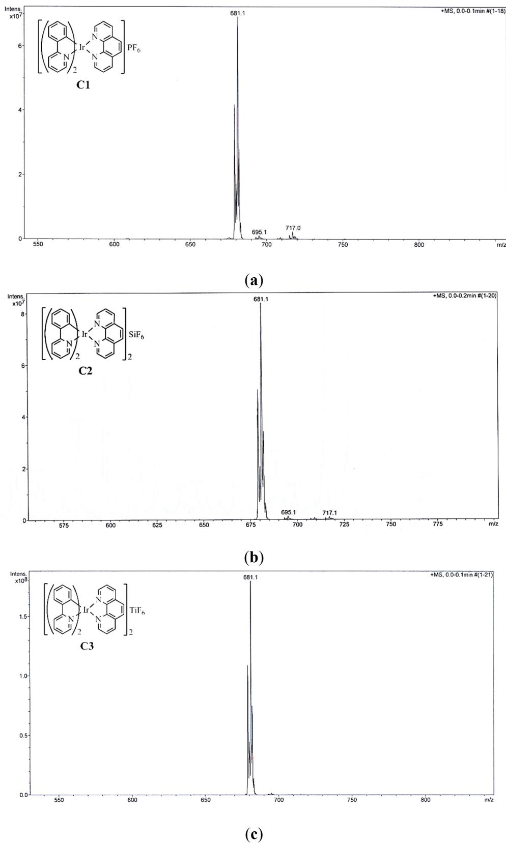
**Figure S1.** Mass spectra of (a)  $[\text{Ir}(\text{ppy})_2(\text{phen})]\text{PF}_6$  (C1); (b)  $[\text{Ir}(\text{ppy})_2(\text{phen})]_2\text{SiF}_6$  (C2); and (c)  $[\text{Ir}(\text{ppy})_2(\text{phen})]_2\text{TiF}_6$  (C3).
