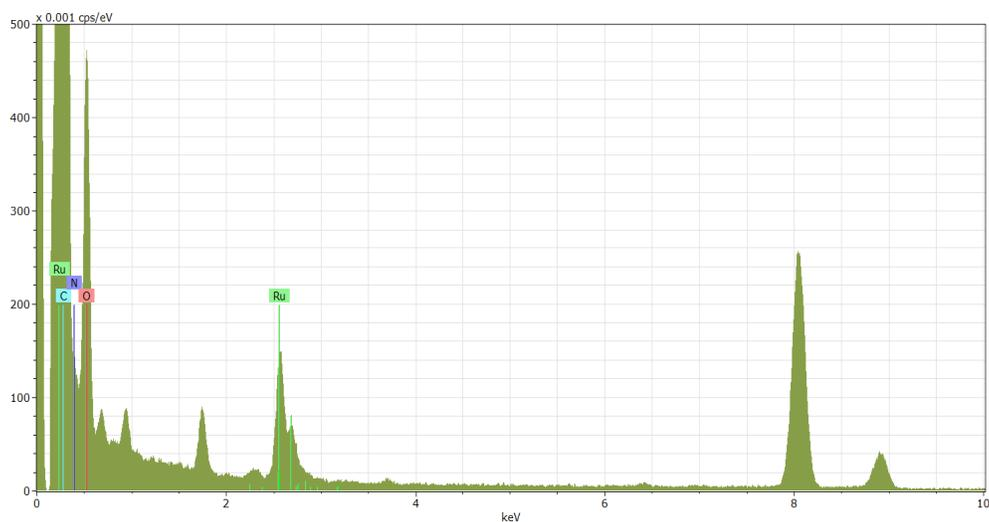
**Figure S5.** The EDX spectrum of the spent Ru-C catalyst after the long-term stability test (80 h).
