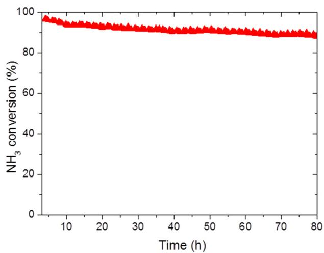
**Figure S4.** Long term stability for NH<sub>3</sub> dehydrogenation over Ru-N-C at 550 °C with a GHSV of 7448 mL·g<sup>-1</sup>·h<sup>-1</sup>.
