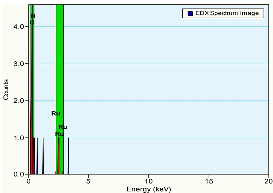
**Figure S1.** The EDX spectrum of Ru-N-C.
