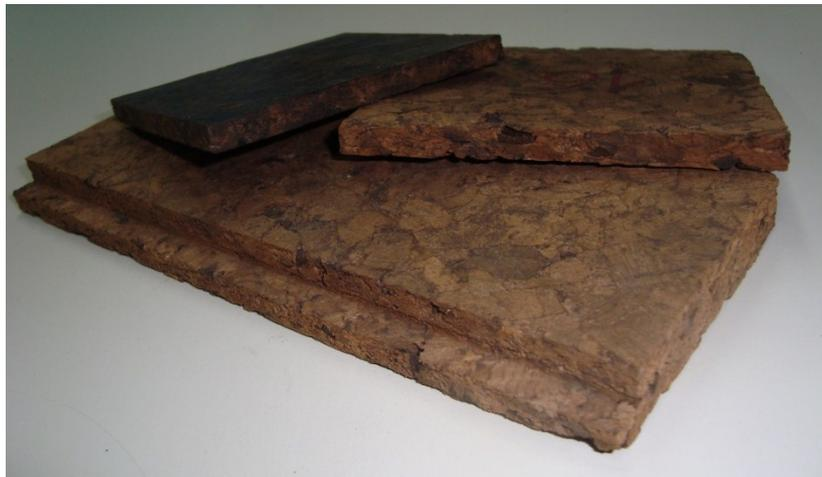
**Figure 1.** Samples of different densified insulation corkboard (ICB) materials.
