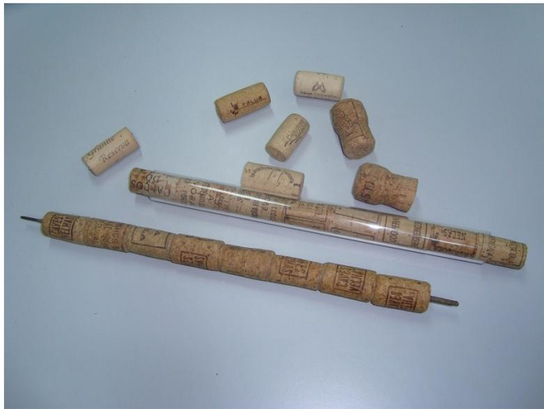
**Figure 4.** Batons of used cork stoppers.
