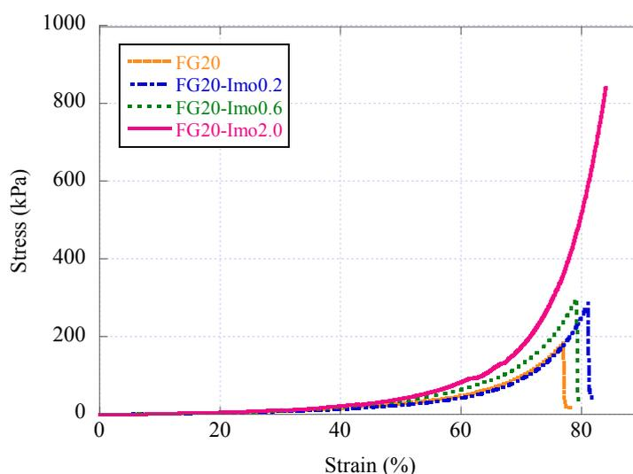
Figure 6a,b shows the results of stress-strain curves in the compression tests of FG10 series and FG30 series, respectively. While we observed moderate improvement of compression strength with imogolite for FG10 series, addition of imogolite diminished the compression strength for FG30 series. The compression strength of FG30-imo0.6 was lower than FG30 without imogolite. FG30-imo0.6 was a very brittle gel, and the strain at break of FG30-imo0.6 became low, resulting in lower toughness.
