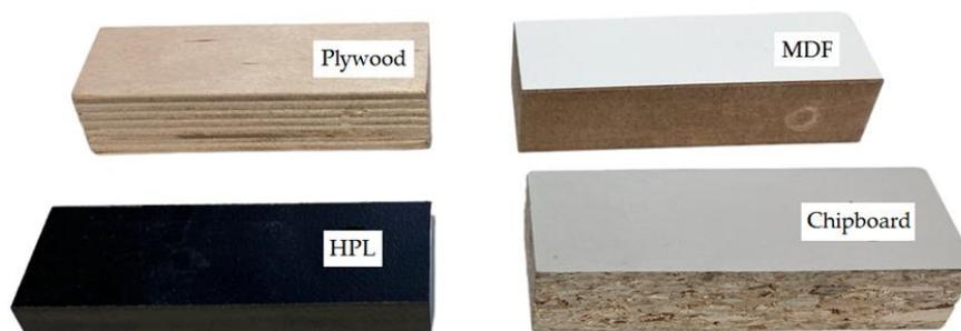
Figure 1. The test materials.
