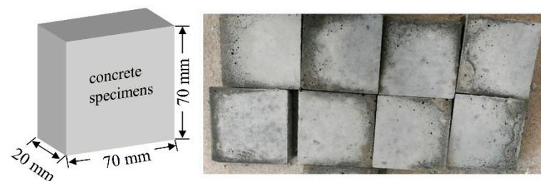
**Figure 2.** Diagram of concrete specimen preparation.
