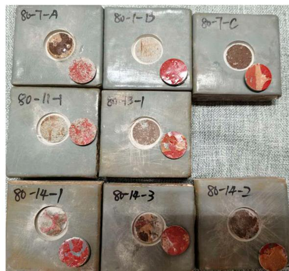
**Figure 10.** The bond failure types of specimens at 80 °C water during the aging test simulated in the tunnel environment.
