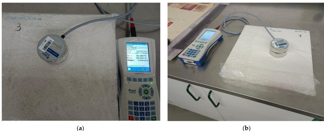
**Figure 3.** Measurements with the MTPS method. (a) Dry material; (b) material after 12 days in the climatic chamber at 80% relative humidity.
