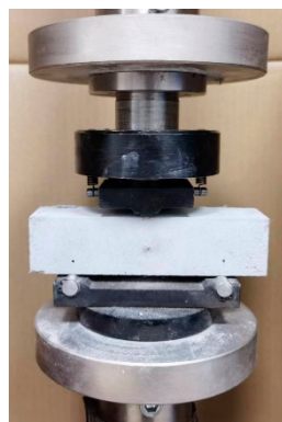
Figure 4. Three-point bending test loading device.
