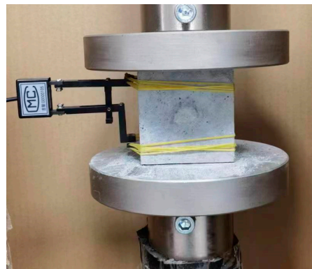
Figure 3. Compressive strength test specimen.
