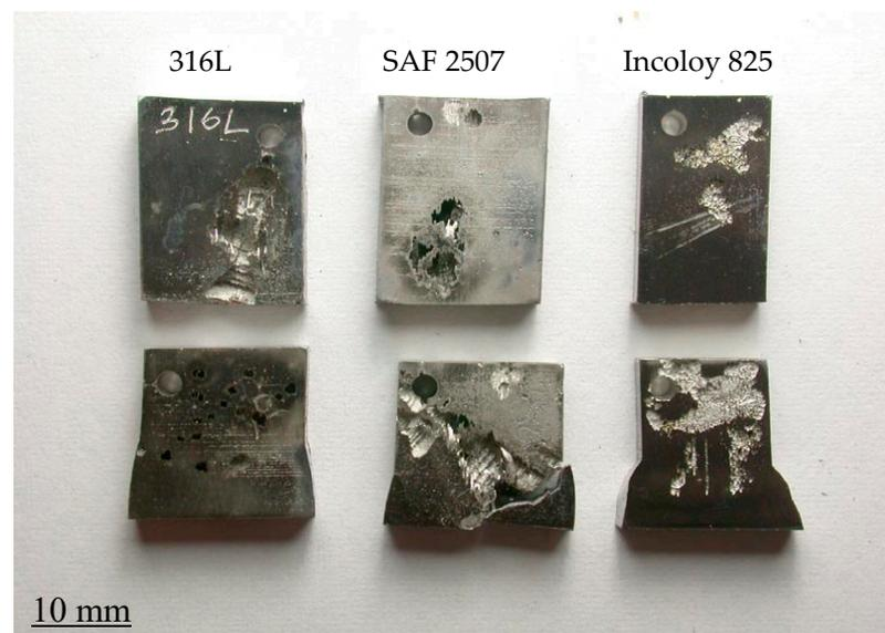
**Figure 9.** Appearance of coupons of parent metals and weldments of SAF 2507 and Incoloy 825 and 316L after exposure to a 6%  $\text{FeCl}_3$  solution (with 7872 ppm nitrite) at 50 °C for 72 h (**Top row:** parent metals; **bottom row:** weldments).
