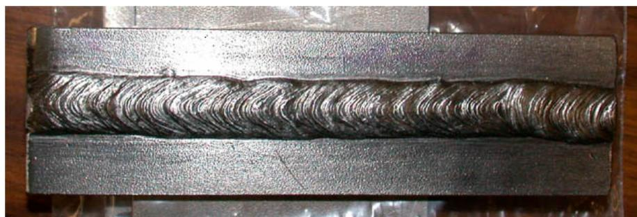
**Figure 1.** Weld plate ready for machining into rectangular weldment specimens.
