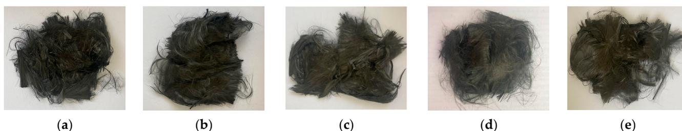
**Figure 4.** Samples after the solvolysis experiments ((a) for the Experiment #01 operating conditions, (b) for the Experiment #02 operating conditions, (c) for the Experiment #03 operating conditions, (d) for the Experiment #04 operating conditions, (e) for the Experiment #05 operating conditions).
