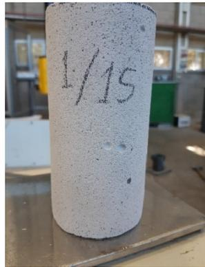
**Figure 6.** Discrete large pores in a highest density specimen.
