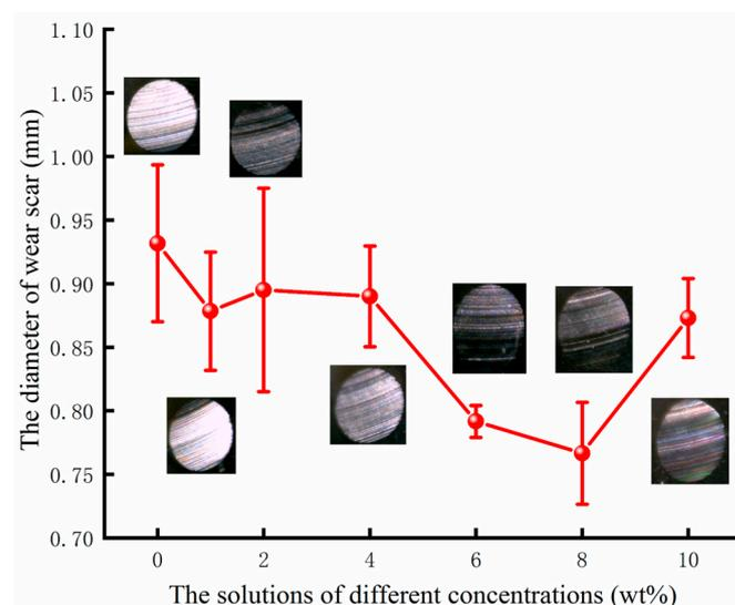
**Figure 7.** The diameter of the wear scar under different lubricants.
