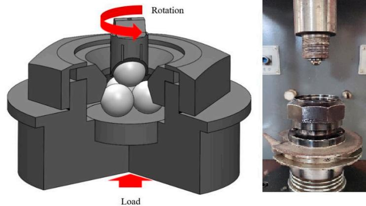
**Figure 2.** Four-ball tribometer [31].
