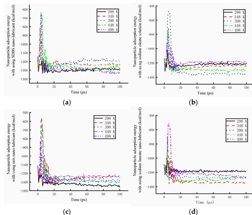
**Figure 15.** The absorption energy of nanoparticles in different lubricants under different working temperatures. (a) Nanoparticle absorption energy in the SDBS lubricant. (b) Nanoparticle absorption energy in the sodium oleate lubricant. (c) Nanoparticle absorption energy in the sodium oleate and sodium laurate lubricant. (d) Nanoparticle absorption energy in the sodium laurate lubricant.
