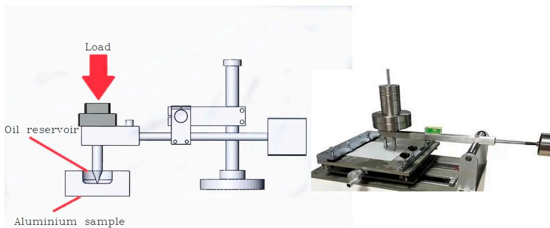
**Figure 3.** Scratch tester.
