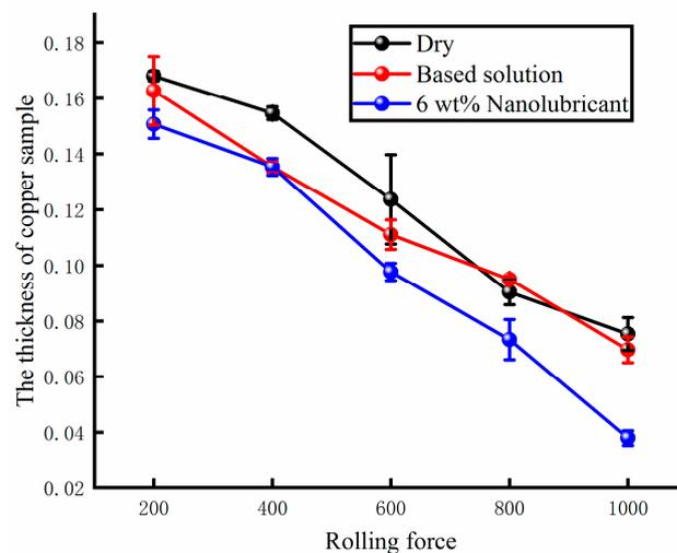
**Figure 16.** The thickness of the rolled Cu samples under different lubricating conditions.
