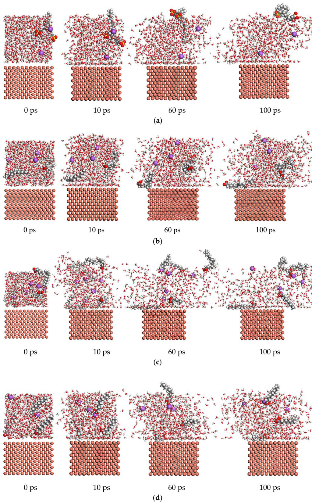
**Figure 11.** The dynamic path molecules of different base solutions. (a) The dynamic path molecules of the base solution mixed with SDBS. (b) The dynamic path molecules of the base solution mixed with sodium oleate. (c) The dynamic path molecules of the base solution mixed with sodium oleate and sodium laurate. (d) The dynamic path molecules of the base solution mixed with sodium laurate.
