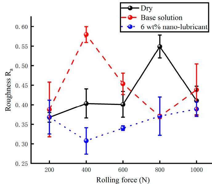
**Figure 17.** The surface roughness  $R_a$  of rolled strips under different lubricating conditions.
