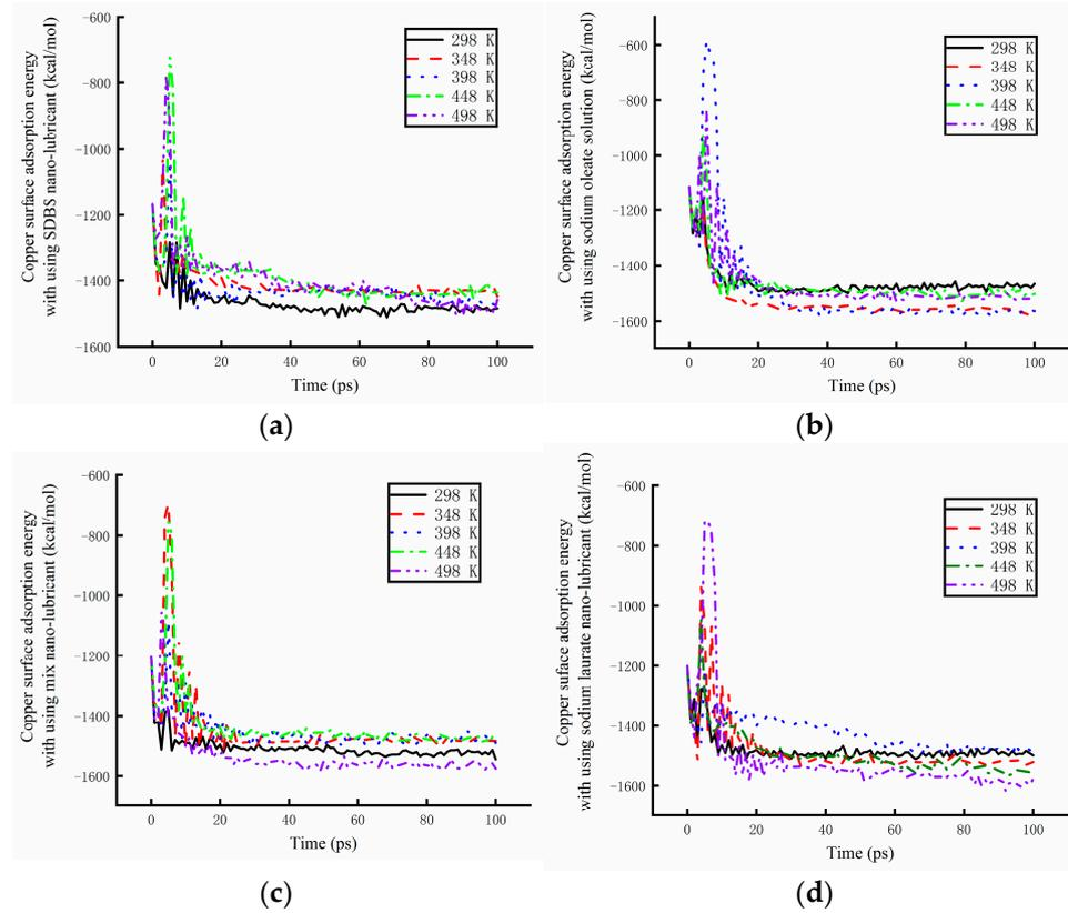
**Figure 13.** The absorption energy of different lubricants mixed with  $Fe_3O_4$  nanoparticles. (a) Absorption energy of the SDBS nanolubricant. (b) Absorption energy of the sodium oleate nanolubricant. (c) Absorption energy of the mix nanolubricant. (d) Absorption energy of the sodium oleate nanolubricant.
