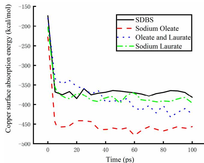
**Figure 10.** The absorption energy of base solutions following addition of different surfactants.
