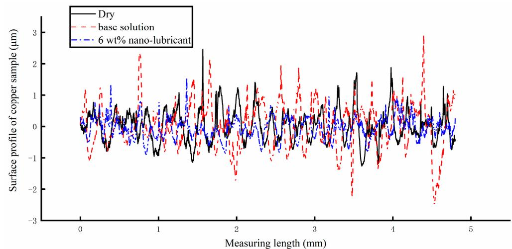
**Figure 18.** The surface profile of the rolled Cu strips under different lubricating conditions.
