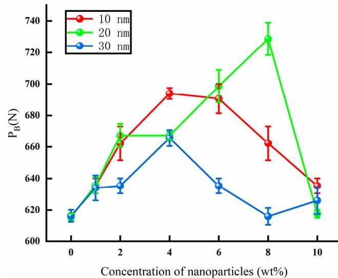
**Figure 5.** The maximum non-seizure load of lubricants ( $P_B$ ) under different concentrations of mixed particles.
