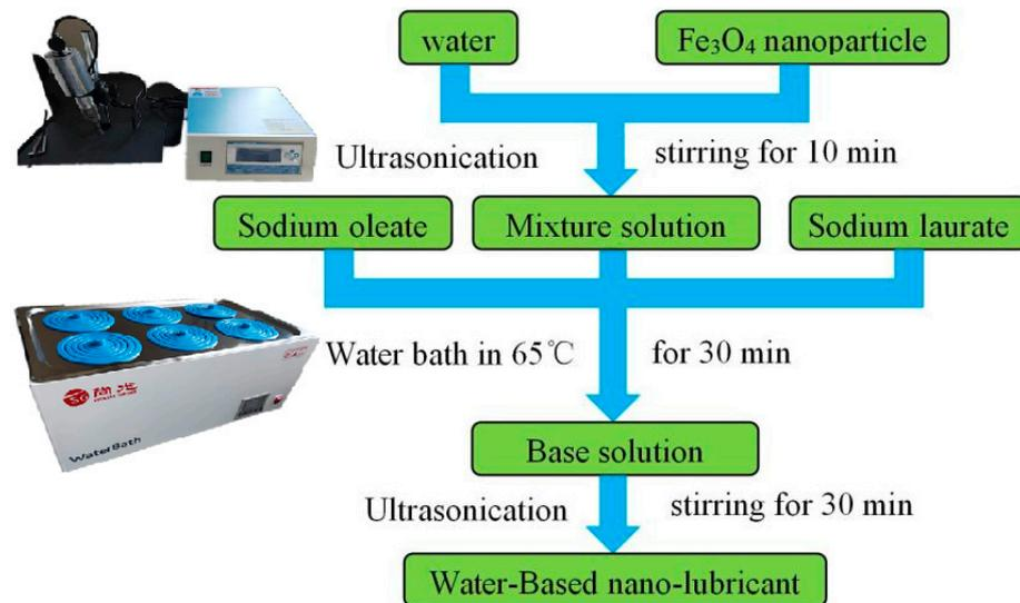
**Figure 1.** The preparation of water-based nanolubricants.
