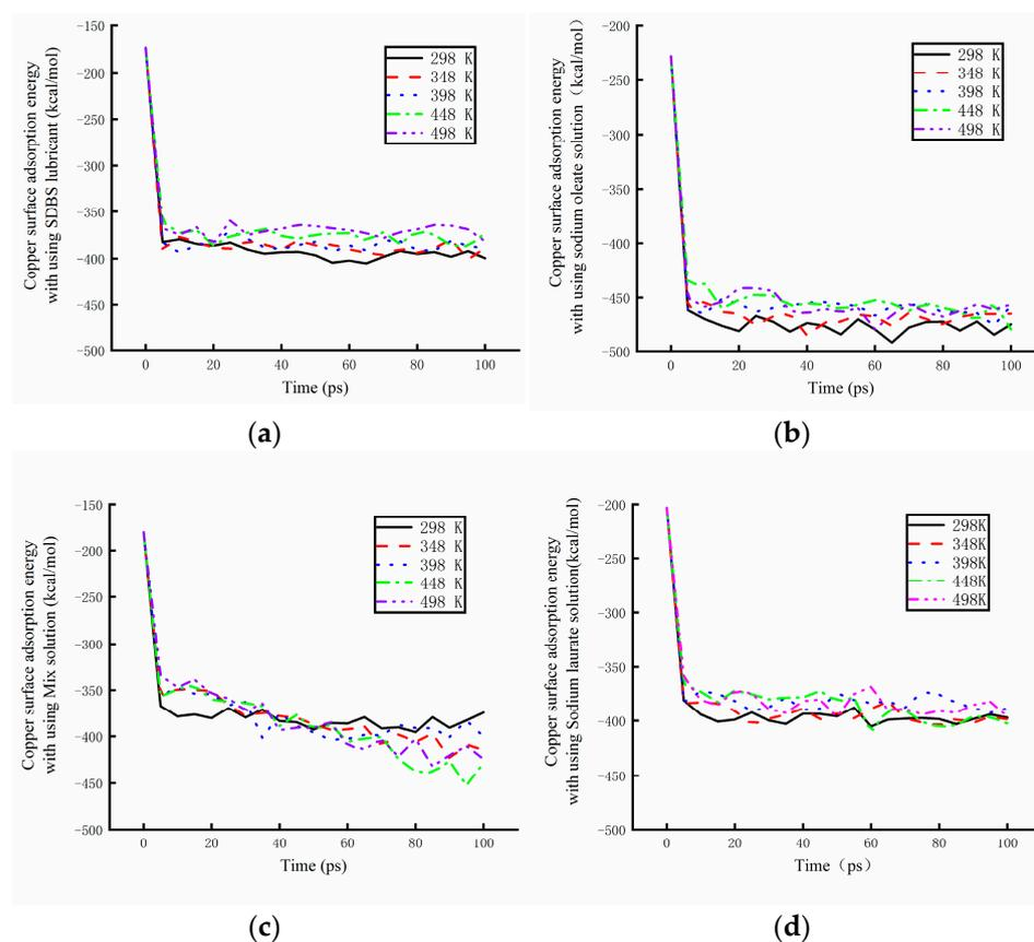
**Figure 12.** The absorption energy of different base solutions under different working temperatures. (a) Absorption energy of the SDBS solution. (b) Absorption energy of the sodium oleate solution. (c) Absorption energy of the mix solution. (d) Absorption energy of the sodium laurate solution.
