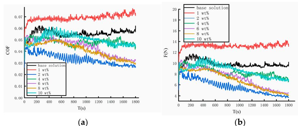
**Figure 6.** The coefficients of friction and friction force during the long-time test. (a) Coefficients of friction. (b) Friction force.
