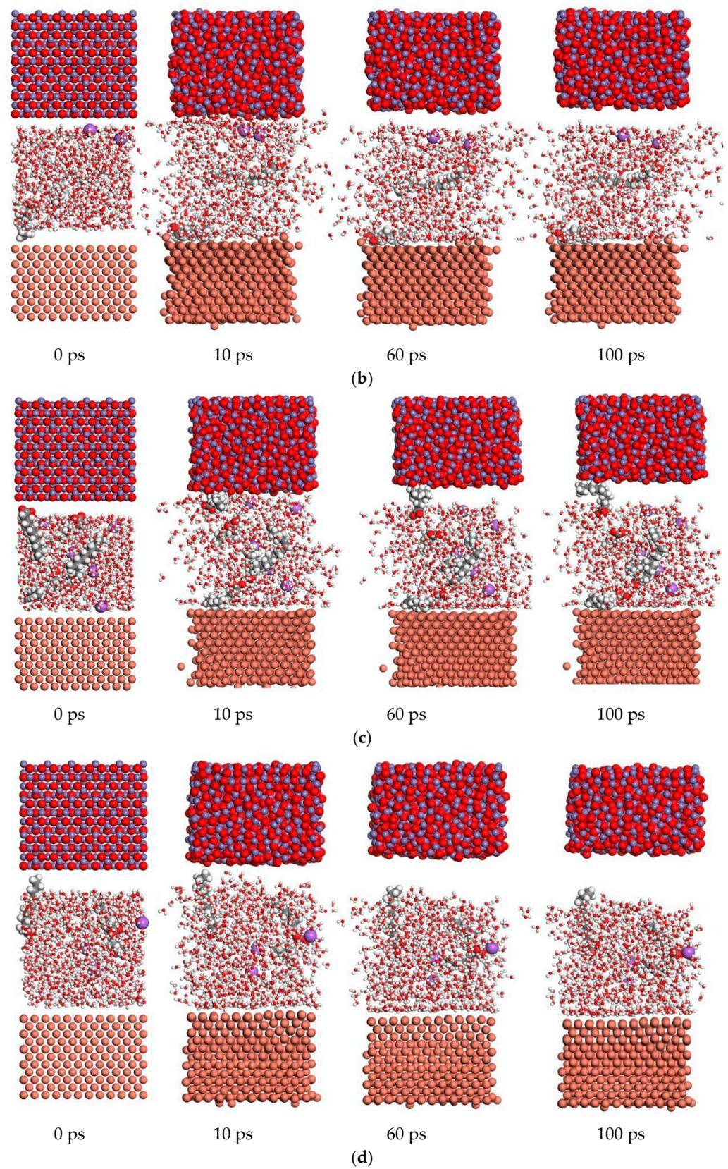
**Figure 14.** The dynamic molecule positions for different lubricants at different times. (a) The dynamic molecule positions of the SDBS nanolubricant. (b) The dynamic molecule positions of the sodium oleate nanolubricant. (c) The dynamic molecule positions of the mixed nanolubricant. (d) The dynamic molecule positions of the sodium laurate nanolubricant.
