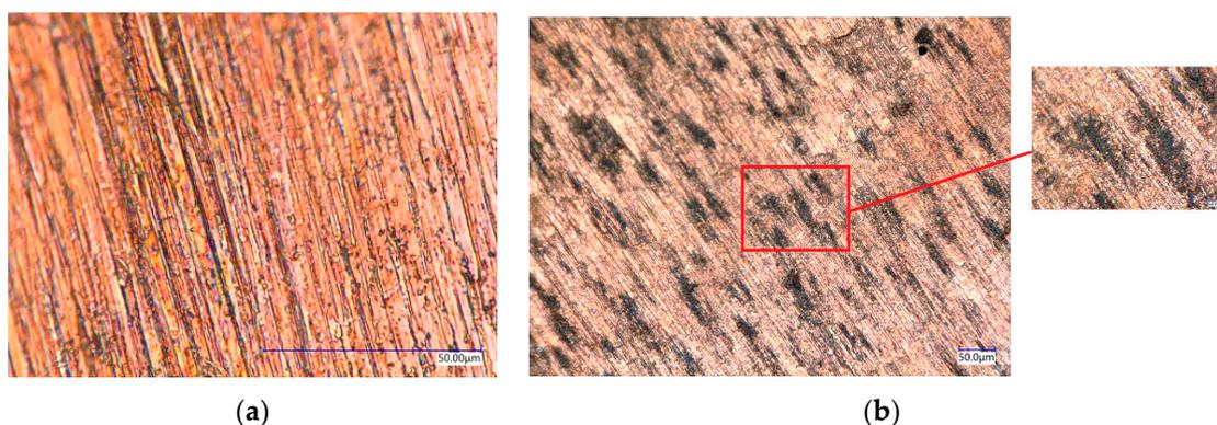
**Figure 19.** The surface morphology of the rolled samples under different lubricating conditions. (a) Surface morphology of Cu samples in the absence of lubricants. (b) Surface morphology of Cu samples using the 6 wt% water-based lubricant.
