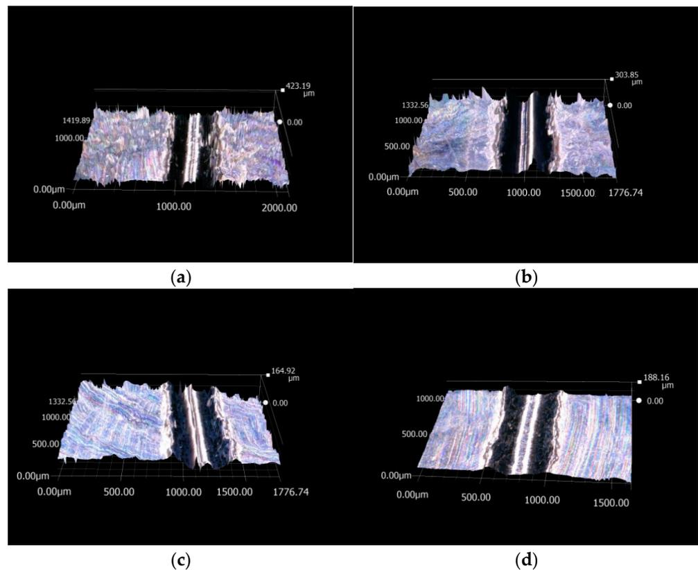
**Figure 9.** The morphology of the scratch under different lubricating conditions. (a) Dry friction condition. (b) Base solution. (c) Water-based nanolubricant (6 wt%). (d) Water-based nanolubricant (8 wt%).
