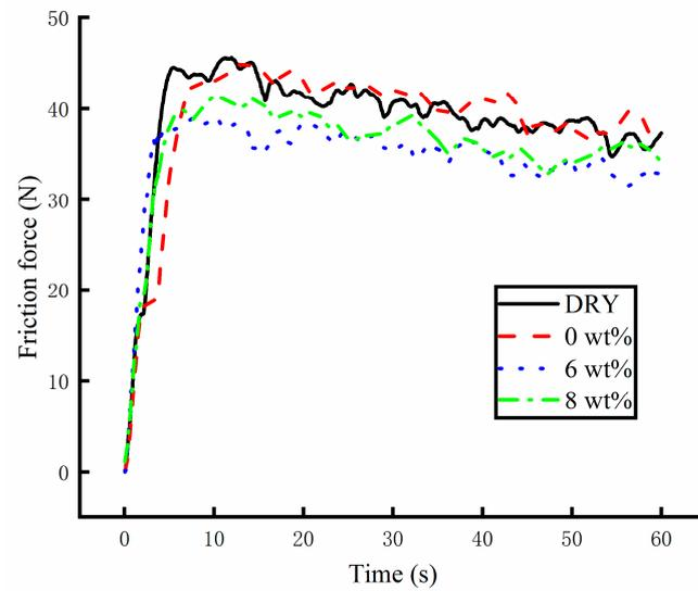
**Figure 8.** The friction force recorded during the scratch test under different lubricating conditions.
