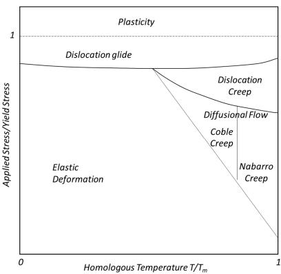
**Figure 2.** Generic deformation mechanism map.
