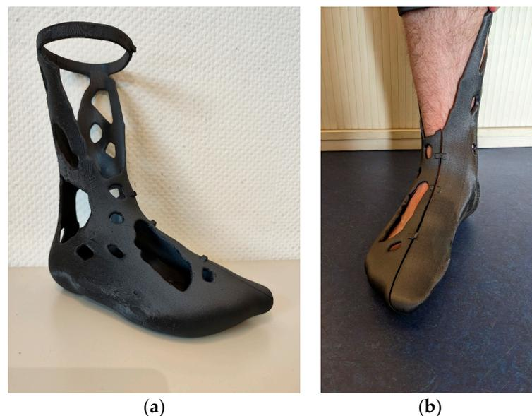
**Figure 16.** Finished topology-optimized PETG-CF15 leg splint: (a) perspective view; (b) tightened on the right foot.
