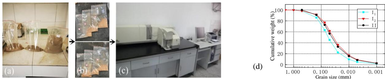
**Figure 5.** Particle size distribution test of soil sample. (a) Sandbagging at 0.075~2 mm; (b) fine particles less than 0.075 mm were packed separately; (c) laser particle size analyzer; (d) gradation curve of soil samples.
