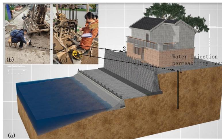
**Figure 20.** On-site water-injection permeability test. (a) Arrangement of water-injection holes; (b) water-injection test for hole 1; (c) water-injection test for hole 2.
