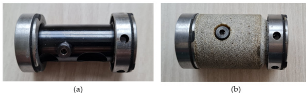
Figure 2. Tested rotor casings: (a) original RC_0; (b) RC_3 with polymer composite filled with silica sand.
