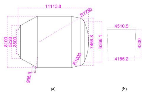
Figure 1. Geometric of the (a) converter; (b) ladle.
