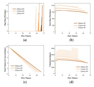
**Figure 9.** The variation trend of (**a**) slag mass flow; (**b**) steel mass flow; (**c**) steel volume in converter, and (**d**) tapping velocity with flowing time when the tilting hole sizes of the converter are 200 mm, 210 mm, or 220 mm.
