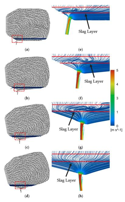
**Figure 6.** Velocity vector diagram at converter angles (**a**)  $90^{\circ}$ , (**b**)  $95^{\circ}$ , (**c**)  $100^{\circ}$ , (**d**)  $105^{\circ}$ , and streamlines diagram at angles (**e**)  $90^{\circ}$ , (**f**)  $95^{\circ}$ , (**g**)  $100^{\circ}$ , (**h**)  $105^{\circ}$ .
