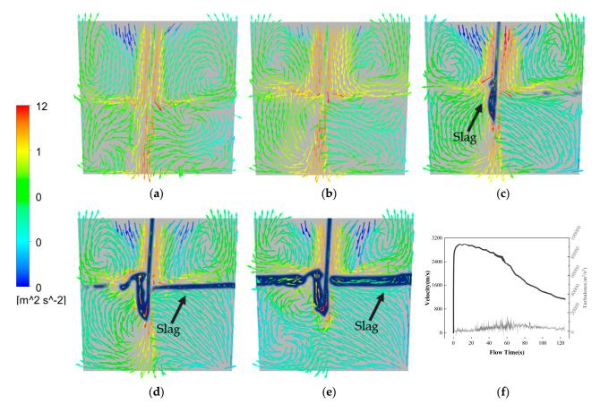
**Figure 4.** Turbulent flow distribution diagram in the ladle at (**a**) 20 s; (**b**) 50 s; (**c**) 70 s; (**d**) 90 s; (**e**) 125 s during steel tapping when the converter is at  $90^{\circ}$  and (**f**) velocity vector and turbulence intensity distribution.
