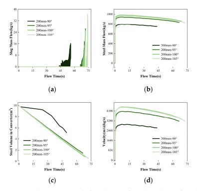
**Figure 7.** The variation trend of (**a**) slag mass flow; (**b**) steel mass flow; (**c**) steel volume in converter and (**d**) tapping velocity with flowing time when the tilting angle of the converter is  $90^{\circ}$ ,  $95^{\circ}$ ,  $100^{\circ}$ , or  $105^{\circ}$ .
