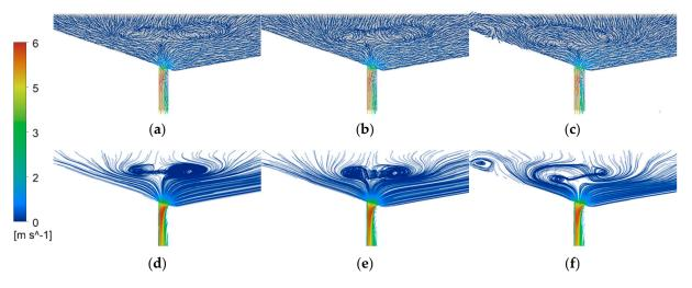
**Figure 10.** Velocity vector distribution of converter tapping hole with diameters of (**a**) 200 mm, (**b**) 210 mm, and (**c**) 220 mm, as well as (**d**) 200 mm, (**e**) 210 mm, and (**f**) 220 mm velocity streamlines distribution.
