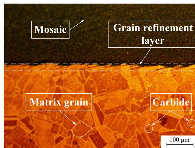
**Figure 11.** Metallographic structure of the GH4169 workpiece cross-section.
