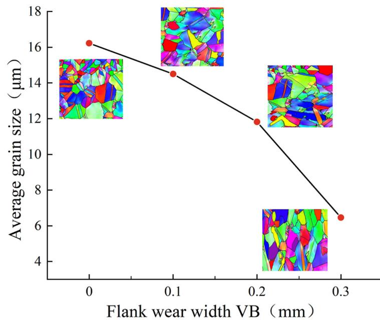
Figure 16. Statistics of the grain morphology and average size in the GH4169 cutting metamorphic layer under different flank wears.
