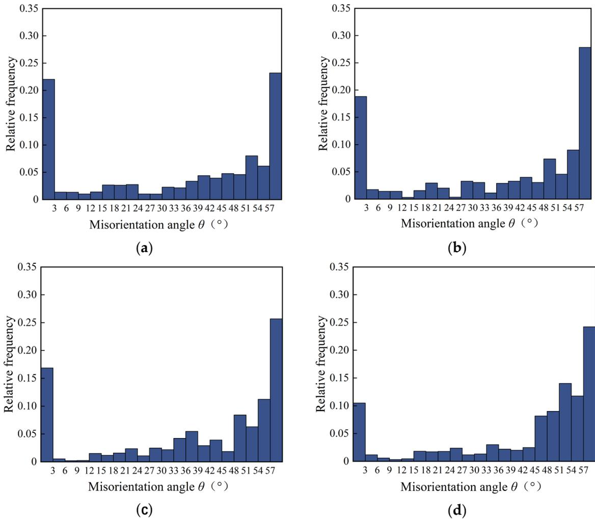
**Figure 18.** Distribution of grain boundary misorientation in the metamorphic layer of the GH4169 cutting surface under different flank wears: (a) VB = 0 mm; (b) VB = 0.1 mm; (c) VB = 0.2 mm; (d) VB = 0.3 mm.
