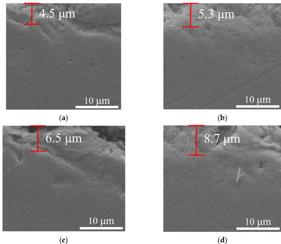
**Figure 14.** Influence of flank wear on metamorphic layer thickness under high-pressure cooling: (a) VB = 0 mm; (b) VB = 0.1 mm; (c) VB = 0.2 mm; (d) VB = 0.3 mm.
