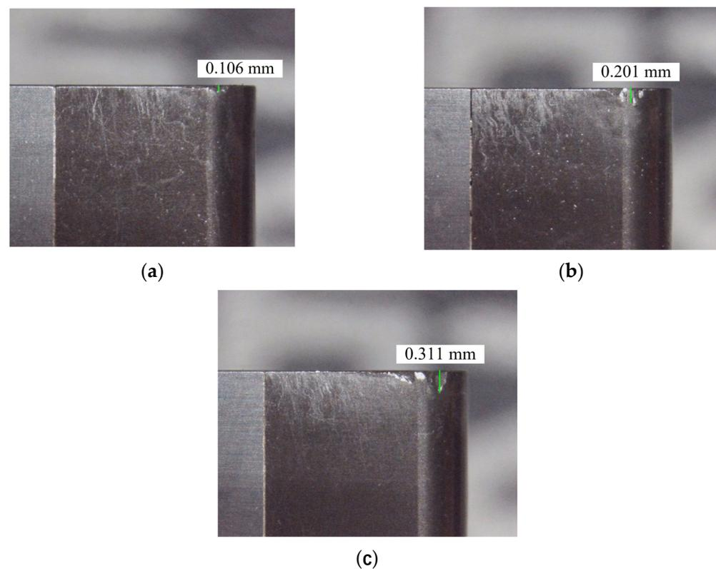
**Figure 8.** Pre-ground PCBN tool: (a) VB = 0.1 mm; (b) VB = 0.2 mm; (c) VB = 0.3 mm.
