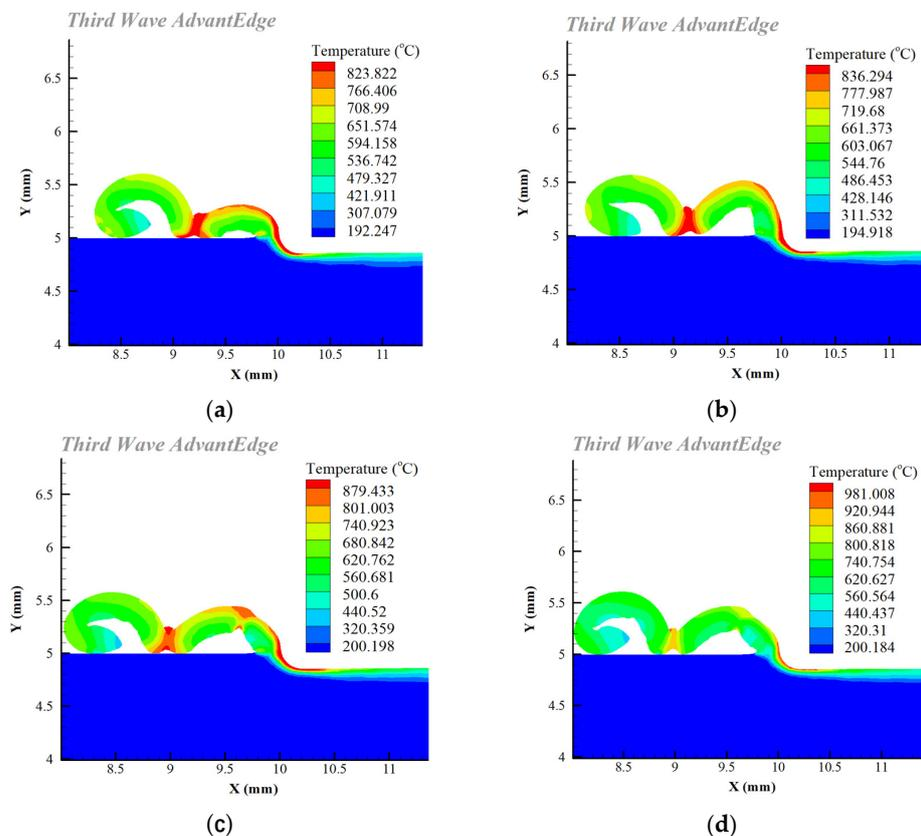
Figure 4. Simulation results for cutting temperature: (a) VB = 0 mm; (b) VB = 0.1 mm; (c) VB = 0.2 mm; (d) VB = 0.3 mm.
