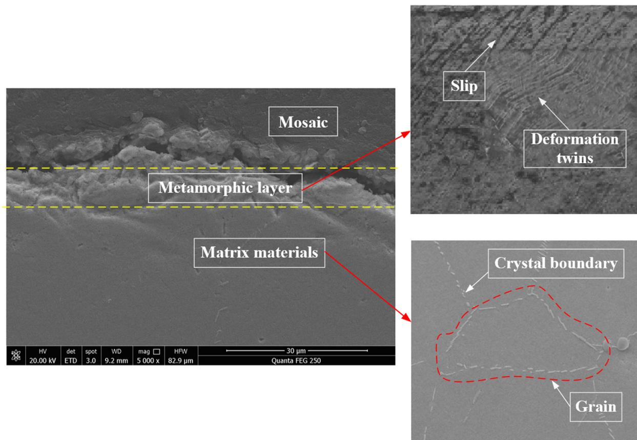
**Figure 13.** The cross-sectional microstructure of the GH4169 workpiece.
