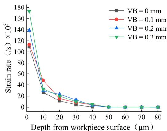
Figure 7. Strain rate in the depth direction of the workpiece surface.
