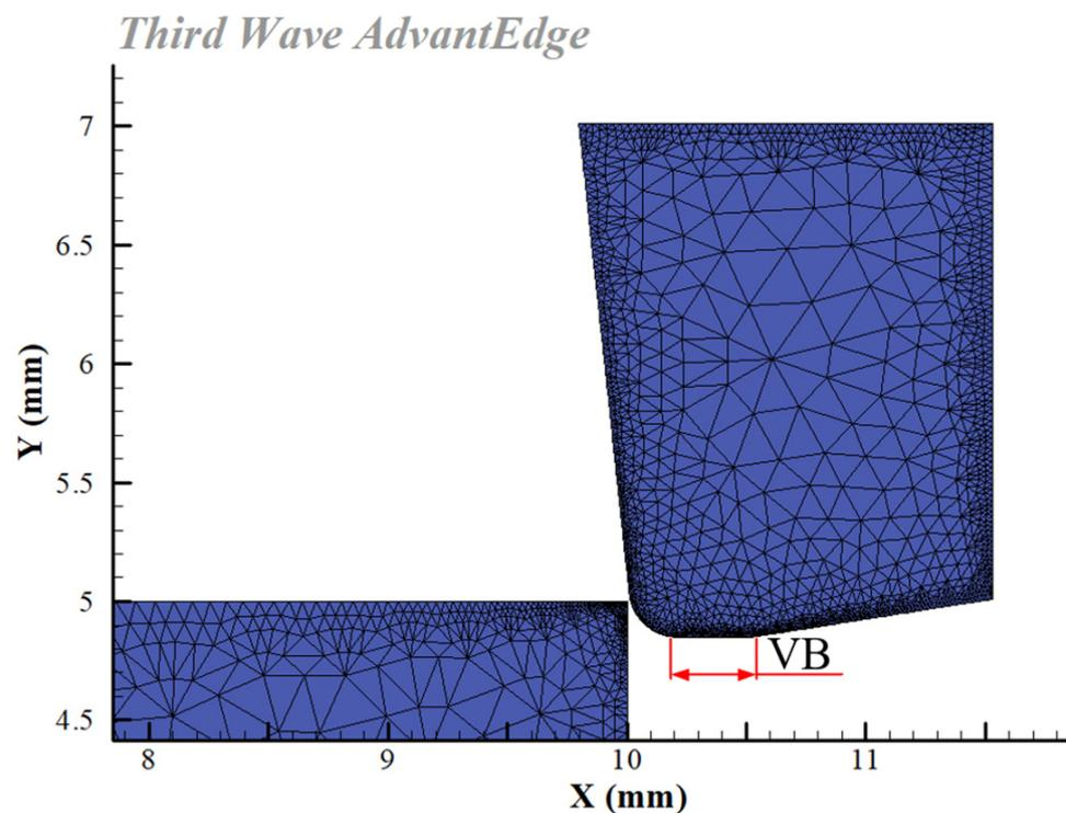
Figure 2. Two-dimensional simulation model of cutting GH4169.
