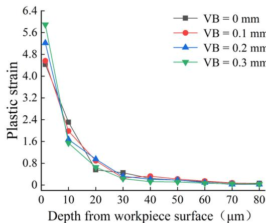
Figure 6. Plastic strain through the depth of workpiece surface.
