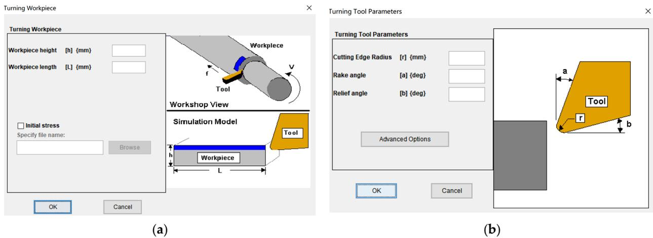
Figure 1. Workpiece–tool parameter settings: (a) standard workpiece; (b) standard tool.
