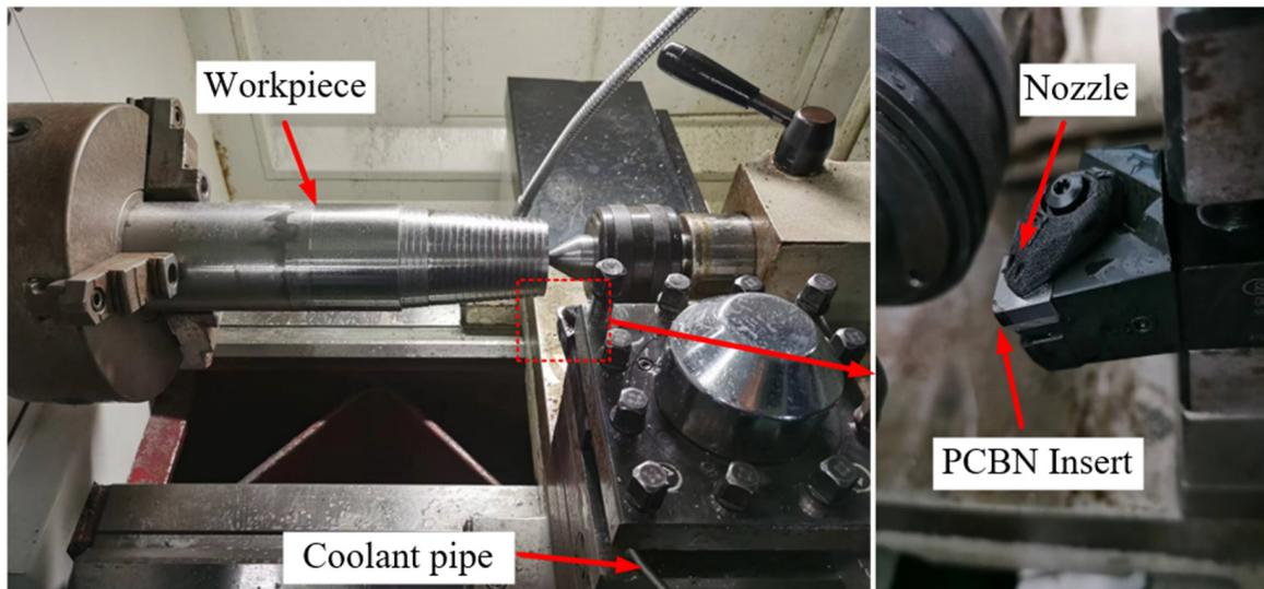
**Figure 9.** Experimental device for cutting GH4169 under high-pressure cooling.
