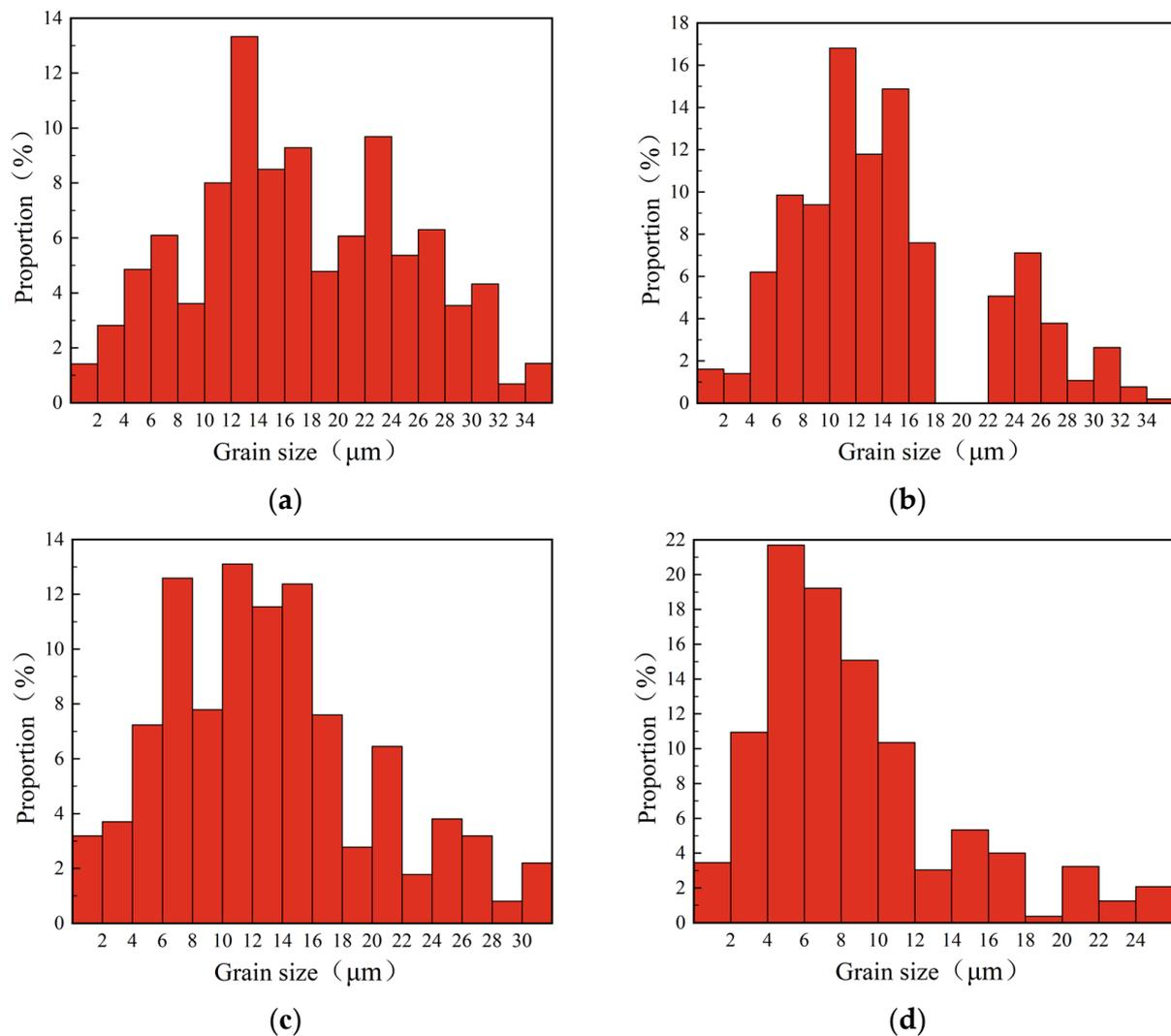
**Figure 17.** Grain size distribution in the metamorphic layer of GH4169 cutting surface under different flank wears: (a) VB = 0 mm; (b) VB = 0.1 mm; (c) VB = 0.2 mm; (d) VB = 0.3 mm.
