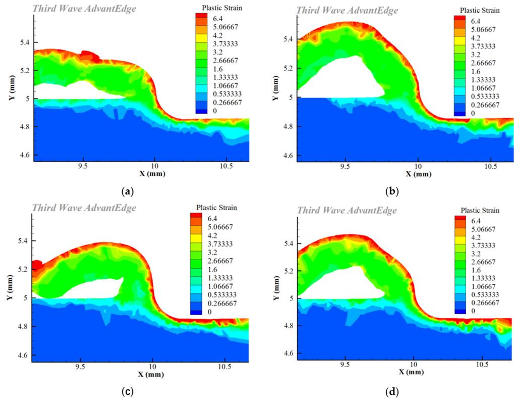
Figure 5. Simulation results for plastic strain: (a) VB = 0 mm; (b) VB = 0.1 mm; (c) VB = 0.2 mm; (d) VB = 0.3 mm.
