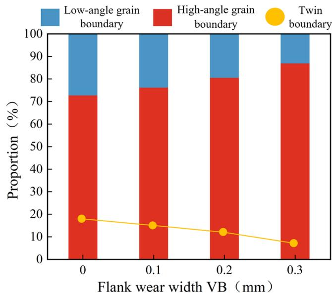
**Figure 19.** Proportion of high-low angle grain boundaries and twin grain boundaries under different flank wears.
