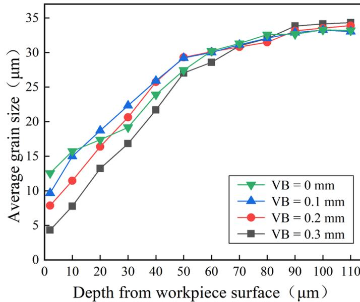
Figure 15. Statistics of the average grain size distribution in the depth direction in the cross-section of the GH4169 workpiece.
