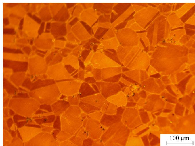
**Figure 12.** Initial microstructure of the GH4169.
