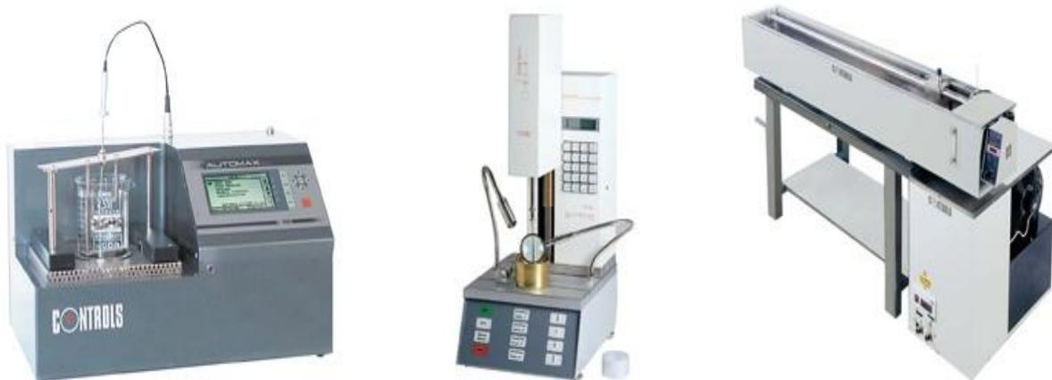
**Figure 2.** Testing devices from left to right—ring and ball, penetration needle, and ductility device.
