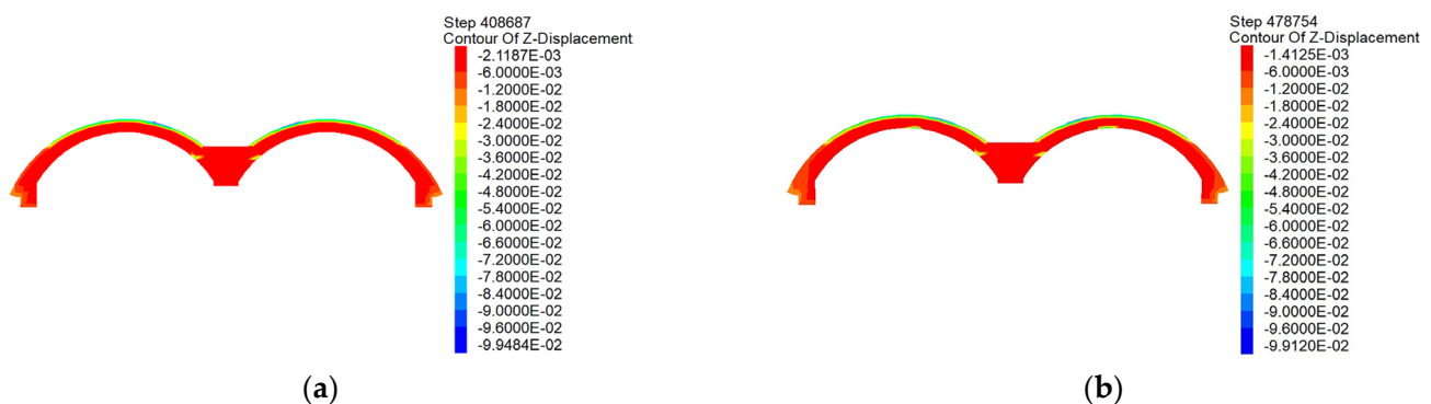
Figure 23. Comparison of the most vertical displacements of the arches completed in (a) one and (b) two attempts.
