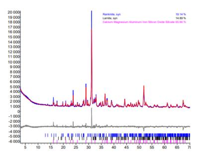
**Figure 9.** Rietveld analysis curve of the product synthesized at 1150  $^{\circ}$ C in 45 min from a mixture of Karpenai limestone and Saltiskiai clay with CaO/SiO<sub>2</sub> = 1.5.
