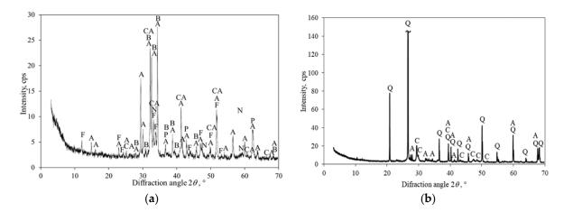
**Figure 12.** XRD patterns of JSC *Akmenes cementas* OPC clinker (a) and after 24 h of carbonization of samples at 45 °C (b). Indexes: A—alite, B—belite, CA—tricalcium alumina, F—calcium aluminum iron oxide, P—periclase, N—sodium calcium aluminum oxide, C—calcite, Q—quartz.
