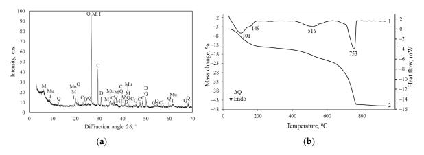
**Figure 4.** XRD pattern (**a**) and STA curves (**b**); 1—DSC, 2—TG of Saltiskiai clay. Indexes: C—calcite, D—dolomite, Q—quartz, I—illite, M—montmorillonite, Ms—muscovite.
