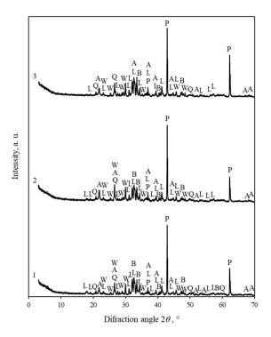
**Figure 11.** XRD patterns of akermanite synthesized for 1 h (1) and after 24 h of carbonization at  $25 \,^{\circ}$ C (2) and  $45 \,^{\circ}$ C (3). Indexes: A—akermanite, Q—quartz, W—wollastonite, L—larnite, B—bredigite, P—periclase.
