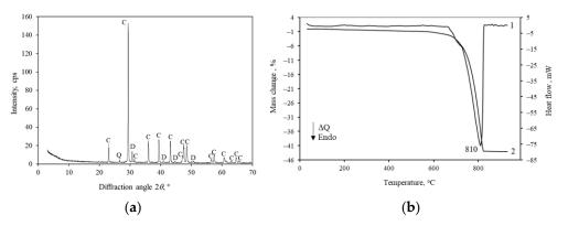
**Figure 2.** XRD pattern (**a**) and STA curves (**b**); 1—DSC, 2—TG of Karpenai limestone. Indexes: C—calcite, D—dolomite, Q—quartz.
