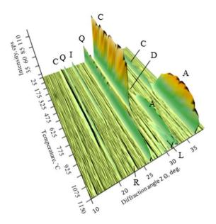
**Figure 6.** XRD diagram of the synthesis product from a mixture of Karpenai limestone and Saltiskiai clay (CaO/SiO<sub>2</sub> = 1.5) in the temperature range of 25–1150  $^{\circ}$ C.
