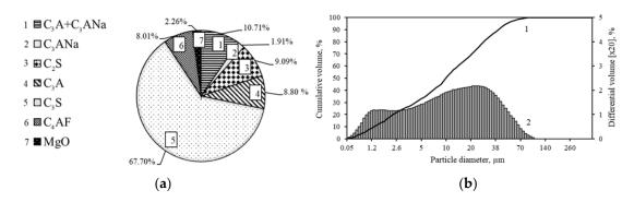
**Figure 5.** Mineralogical (a) and granulometric (b) composition of OPC clinker, where 1—cumulative volume, 2—differential volume. Indexes:  $C_3S$ —alite,  $C_2S$ —belite,  $C_3A$ —calcium aluminum oxide,  $C_3A$ na—sodium calcium aluminum oxide,  $C_4AF$ —calcium aluminum iron oxide, MgO—periclase.
