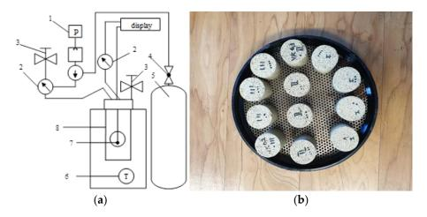
**Figure 1.** Technological system of samples hardening in CO<sub>2</sub> environment (a) and hardened samples (b): 1—pneumatic pump; 2—manometers; 3—shutters; 4—ball valve; 5—CO<sub>2</sub> gas cylinder; 6—temperature sensor; 7—autoclave; 8—heater-thermostat.
