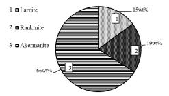
**Figure 10.** Quantitative composition of the synthesis product at  $1150 \,^{\circ}\text{C}$  in 45 min with CaO/SiO<sub>2</sub> = 1.5.
