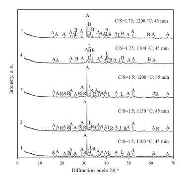
**Figure 7.** XRD patterns of Karpenai limestone—Saltiskiai clay mixtures fired at different temperatures. Indexes: A—akermanite, B—bredigite, R—rankinite, L—larnite.
