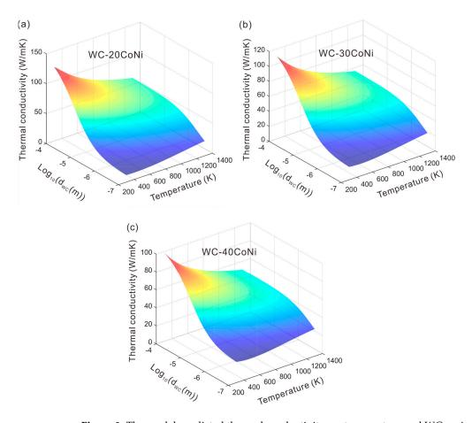
**Figure 9.** The model-predicted thermal conductivity vs. temperature and WC grain size at different phase compositions of: (a) WC-20 wt.% (Co, Ni); (b) WC-30 wt.% (Co, Ni) and (c) WC-40 wt.% (Co, Ni). The composition of (Co,Ni) binder phase is Co–50wt.%Ni.
