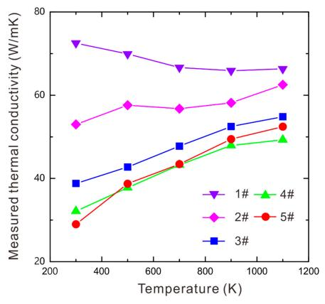
**Figure 5.** Temperature dependence of the measured thermal conductivity of the two-phase WC-Co-Ni samples prepared here.
