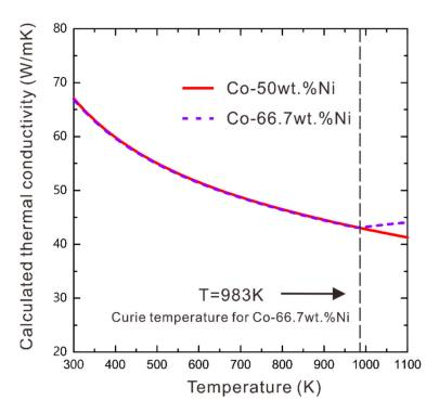
**Figure 6.** Model-evaluated thermal conductivity of Co-50wt.%Ni and Co-66.7wt.%Ni solid solutions along with the temperature.
