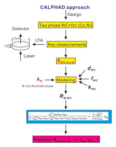
**Figure 1.** The overall strategy of the present work integrating experiments and models.  $k_{WC}$  and  $k_{MC}$  represent thermal conductivity for WC phase and M binder phase, respectively.  $d_{WC}$  represents grain size of WC while  $f_{WC}$  is volume fraction of WC.  $R_{M/WC}$  represents ITR (Interface Thermal Resistance) between the WC phase and the binder phase.
