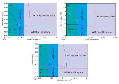
**Figure 2.** Evaluated phase diagrams by Thermo-calc software: (a) WC-30 wt.% (Co, Ni) (Co:Ni = 1:1); (b) WC-40 wt.% (Co, Ni) (Co:Ni = 1:2); and (c) WC-40 wt.% (Co, Ni) (Co:Ni = 1:1).
