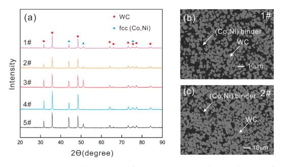
**Figure 4.** (a) XRD patterns of prepared WC-Co-Ni samples; SEM observations for (b) sample 1#; (c) sample 2#.
