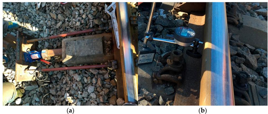
**Figure 4.** Field tests of lateral ballast resistance. (a) Forcing device; (b) Displacement measured by a dial gauge.
