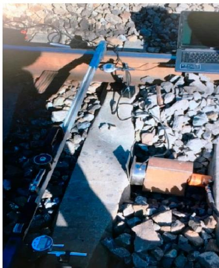
**Figure 2.** Field tests of longitudinal ballast resistance.
