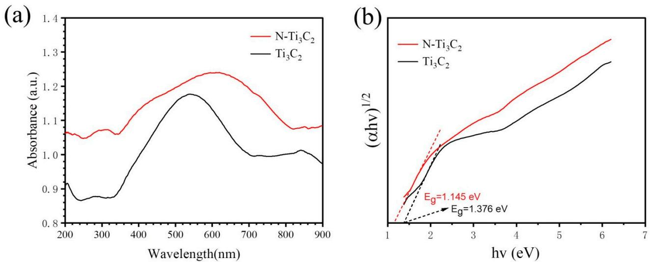
**Figure 9.** (a) Absorption spectra of  $\text{Ti}_3\text{C}_2$  and  $\text{N-Ti}_3\text{C}_2$  samples; (b) plots of  $(\alpha h\nu)^{1/2}$  versus photon energy ( $h\nu$ ) for band-gap energy.
