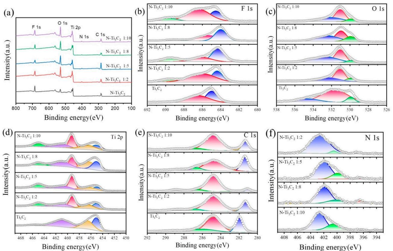
**Figure 5.** XPS spectra of the samples: (a) measurement scan, (b) F 1s, (c) O 1s, (d) Ti 2p, (e) C 1s, (f) N 1 s.
