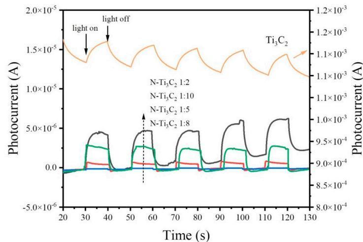
**Figure 6.** Transient photocurrents of  $\text{Ti}_3\text{C}_2$  and  $\text{N-Ti}_3\text{C}_2$  1:8.
