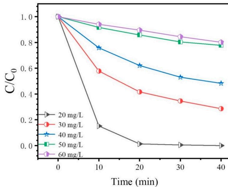
**Figure 8.** Effect of dye concentration on degradation rate.
