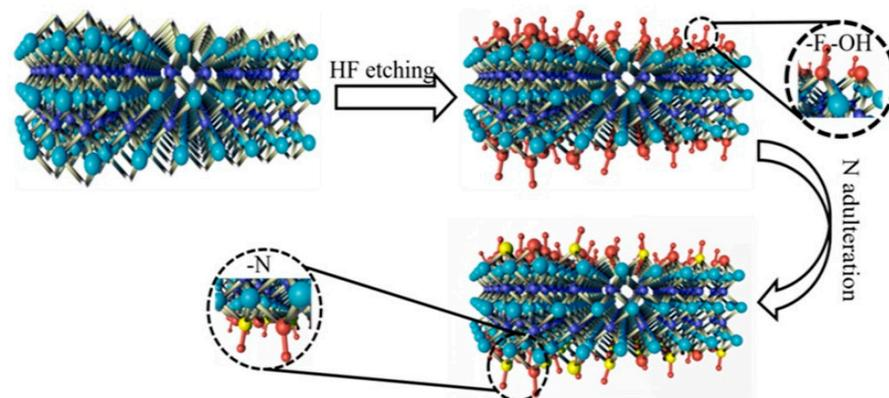
**Figure 2.** Schematic diagram of the synthetic structure of N-Ti<sub>3</sub>C<sub>2</sub> catalyst.
