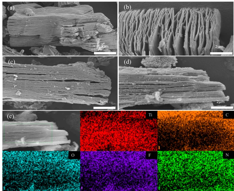
**Figure 3.** (a,b) Local magnifications of layered  $\text{Ti}_3\text{C}_2$  MXene and  $\text{Ti}_3\text{C}_2$ ; (c,d) SEM images of  $\text{N-Ti}_3\text{C}_2$  MXene nanomaterials at different magnifications; (e) EDS elemental mapping of Ti, C, O, F and N nanomaterials of  $\text{N-Ti}_3\text{C}_2$  MXene.
