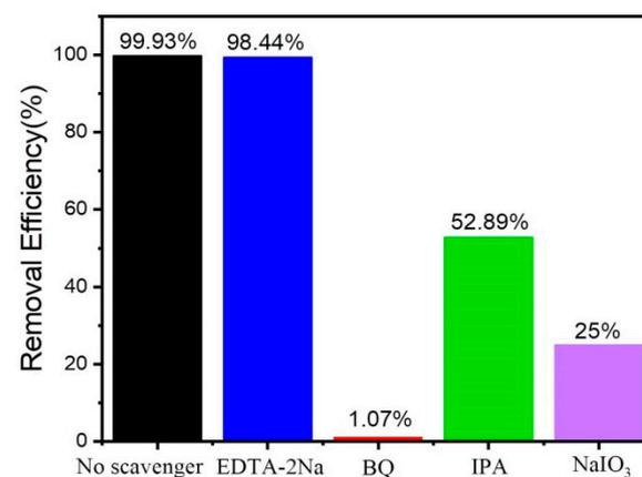
**Figure 10.** Shows the active substance capture experiment for the photo-degradation of MO by  $\text{N-Ti}_3\text{C}_2$  1:8 nanomaterial.
