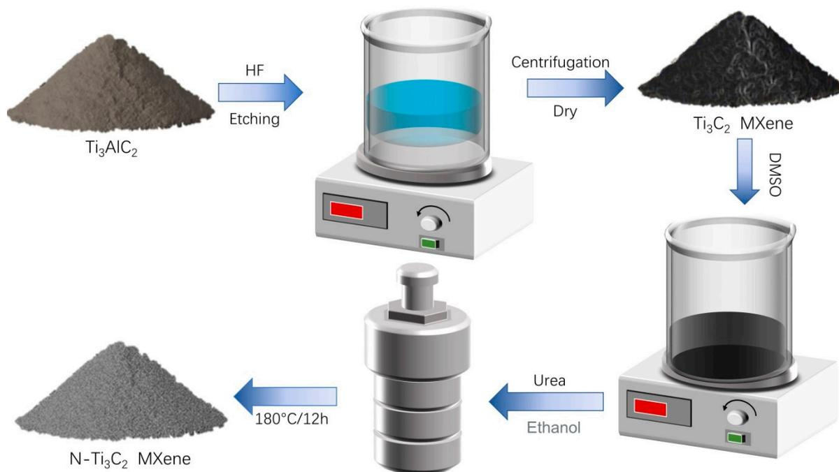
**Figure 1.** Roadmap for the synthesis of N-Ti<sub>3</sub>C<sub>2</sub> catalyst.
