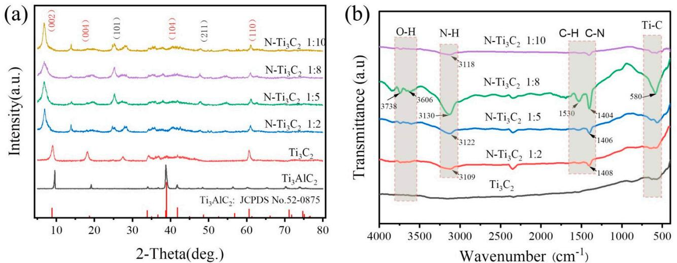
**Figure 4.** (a) XRD patterns of  $\text{Ti}_3\text{C}_2$  MXene and  $\text{N-Ti}_3\text{C}_2$  MXene nanomaterials; (b) FTIR spectra of  $\text{Ti}_3\text{C}_2$  and  $\text{N-Ti}_3\text{C}_2$  MXene.
