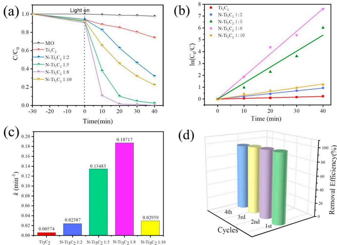
**Figure 7.** Photo-catalytic activity on (a) MO degradation activity, (b) pseudo-level diagram of MO degradation, (c) kinetic constants of MO degradation, (d) reusability of N-Ti<sub>3</sub>C<sub>2</sub> 1:8 for MO degradation.
