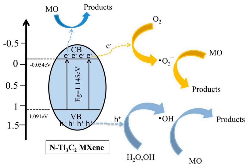
Figure 11. Photocatalytic degradation mechanism of N-Ti<sub>3</sub>C<sub>2</sub> MXene.
