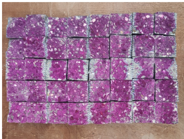
Figure 3. Specimens for carbonation depth testing.
