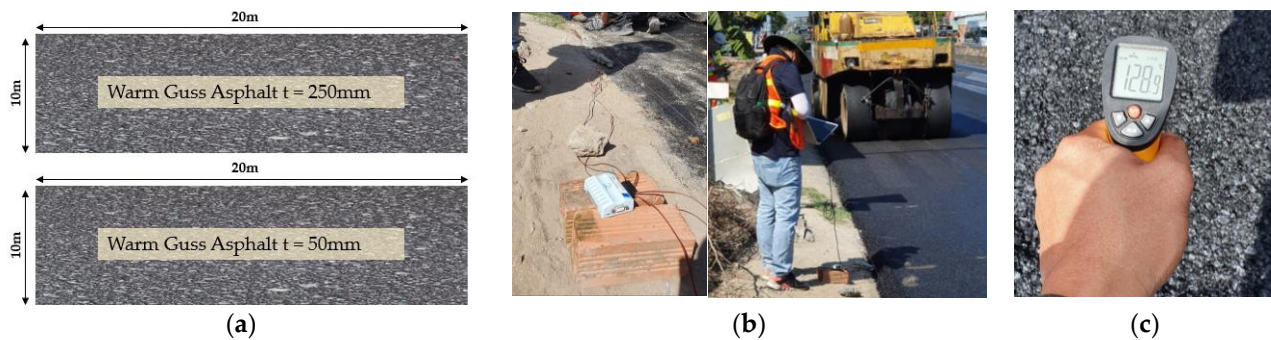
Figure 11. (a) Field testbed section, measurement of the WGA surface by using instrument (b) and thermal meter (c).
