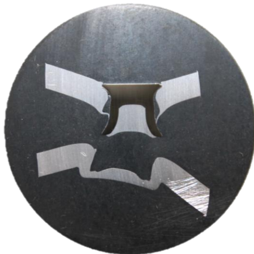
Figure 14. Image of the tail pull-out failure mode experienced in this study.
