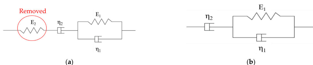
Figure 3. Rheological models: (a) Burgers model; (b) three-element model.
