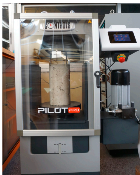
Figure 2. Compression tests on concrete cylinders and results.
