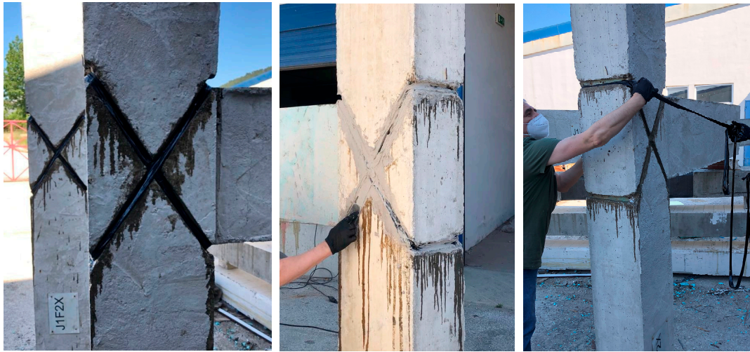
Figure 3. Strengthened specimens CON0F2X, CON1F2X; C-FRP ropes are applied in an X-shape form on the joint body.
