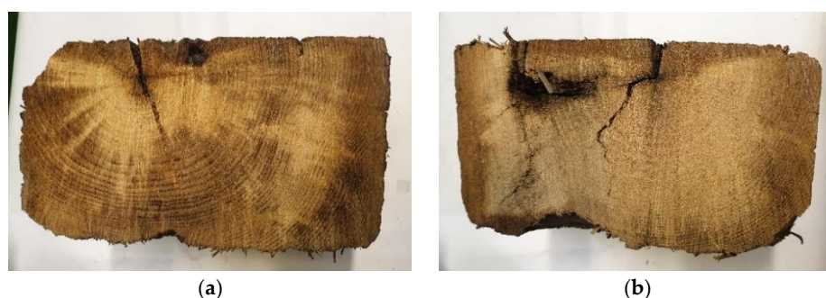
Figure 1. Cross section of the tested tie through the center of length (a) and 1 cm from the edge (b).
