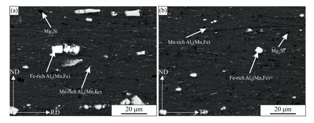
**Figure 3.** The backscattered electron images of the AA 5083-H111 alloy. (a) In the longitudinal direction. (b) In the transverse direction: RD-rolling direction, ND-normal direction, TD-transverse direction.
