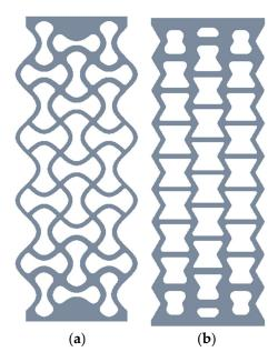
Figure 1. Two examples of cellular structures: (a) chiral structure; (b) re-entrant structure.
