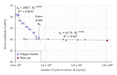
Figure 6. The S-N curve for the rolling direction.
