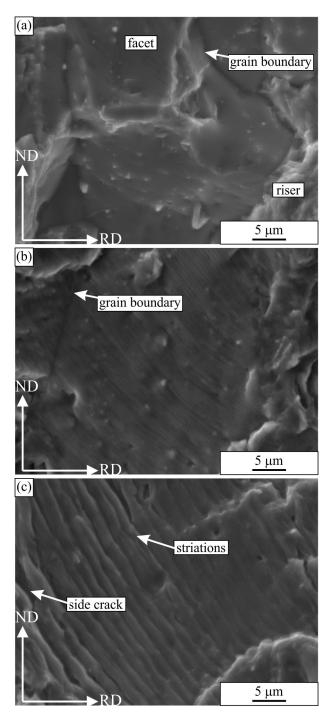
**Figure 12.** Secondary electron micrographs of the fractured surfaces of the fatigue sample PSV 14 (765,121 cycles to failure): (a) 0.7 mm from the fatigue crack initiation (Stage Regime A), (b) 1.4 mm from the fatigue crack initiation (start of Regime B), (c) 3.5 mm from the fatigue crack initiation (near the end of Regime B).
