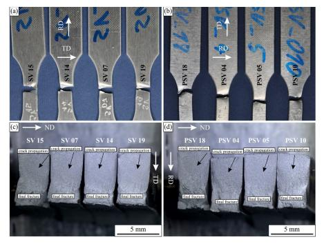
**Figure 9.** The light micrographs of the fractured surfaces of the selected fatigue samples: (a,c) longitudinal layout and (b,d) transverse layout (ND—normal direction, RD—rolling direction, TD—transverse direction).
