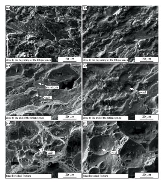
**Figure 11.** The secondary electron micrographs of the fractured surfaces of the fatigue samples tested in the transverse layout: (**a**,**c**,**e**) PSV 18 (135,165 cycles to failure), (**b**,**d**,**f**) SV 10 (15,500,000 cycles to failure). The orientation of all images is the same. The TD direction is perpendicular to the images.
