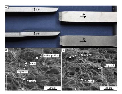
**Figure 5.** The fractured tensile specimens. (a) The photography of the samples. The secondary electron micrographs of the fractured surfaces of the tensile specimens: (b) in the RD and (c) in the TD.
