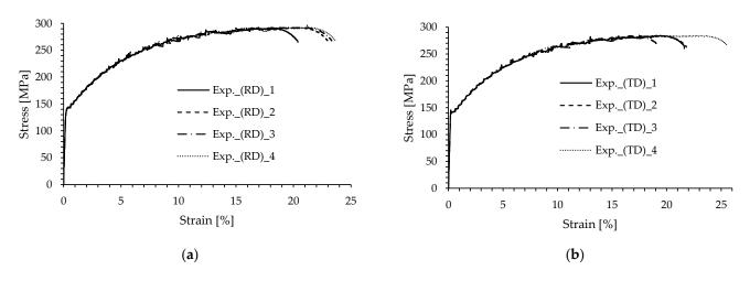
**Figure 4.** Engineering stress–strain curves of the AA 5083-H111 alloy. (a) Rolling direction (RD). (b) Transverse direction (TD).
