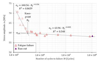
**Figure 7.** The S–N curve for the transverse direction.
