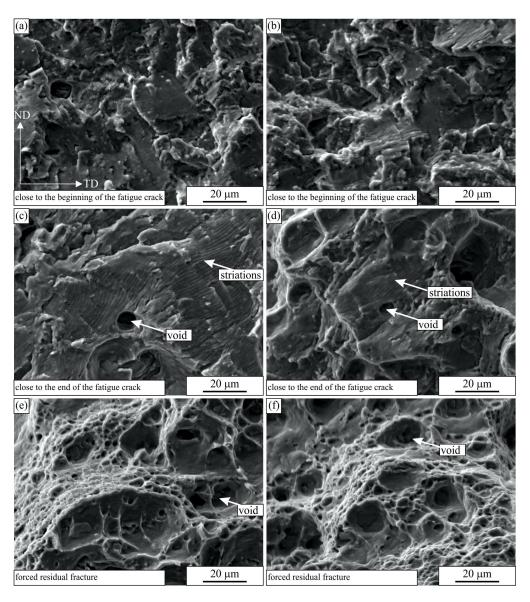
**Figure 10.** The secondary electron micrographs of the fractured surfaces of the fatigue samples tested in the longitudinal layout: (**a**,**c**,**e**) SV 15 (131,581 cycles to failure), (**b**,**d**,**f**) SV 19 (19,392,180 cycles to failure). The orientation of all images is the same. The RD direction is perpendicular to the images.
