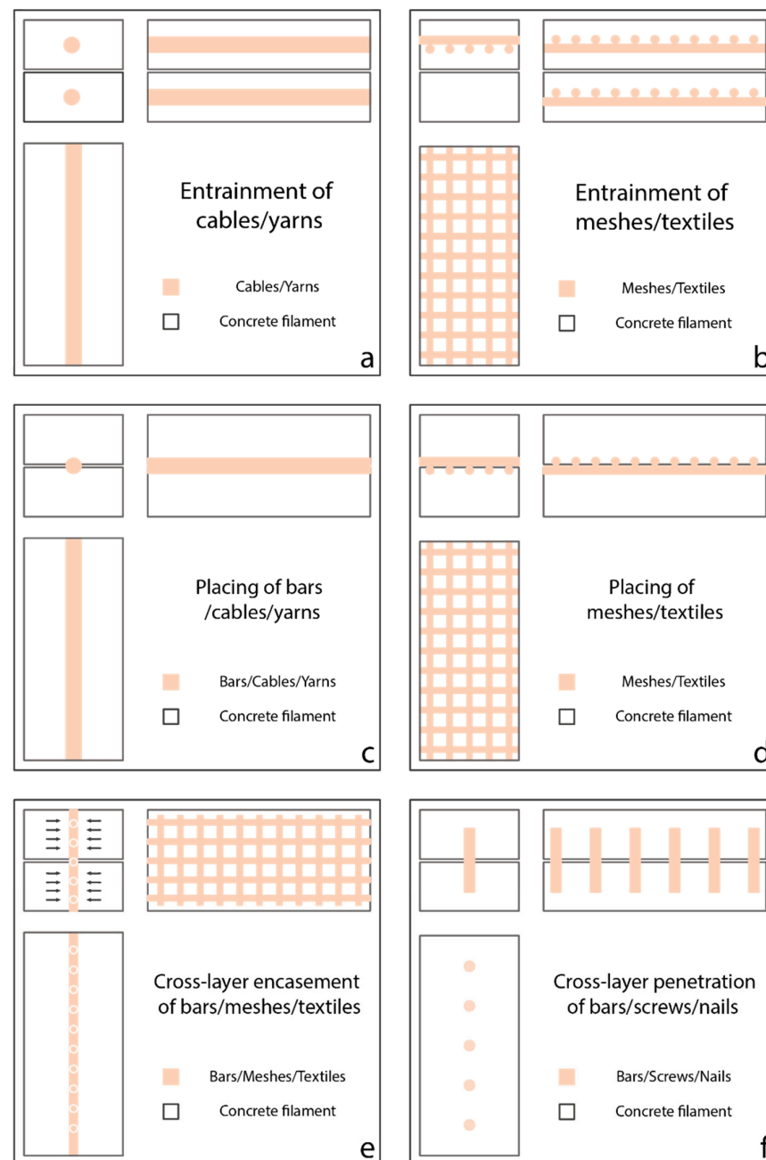
Figure 9. Cross-section view (left-top), side view (right-top) and plan view (left-bottom) of: (a) entrainment of cables/yarns; (b) entrainment of meshes/textiles; (c) placing of bars/cables/yarns; (d) placing of meshes/textiles; (e) cross-layer encasement of bars/meshes/textiles; and (f) cross-layer penetration of bars/screws/nails.
