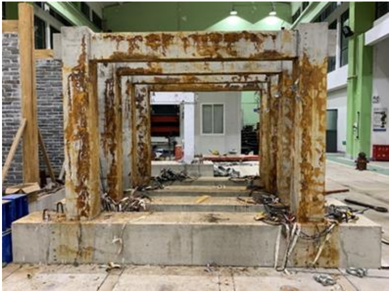
Figure 6. Appearance of corroded specimen.
