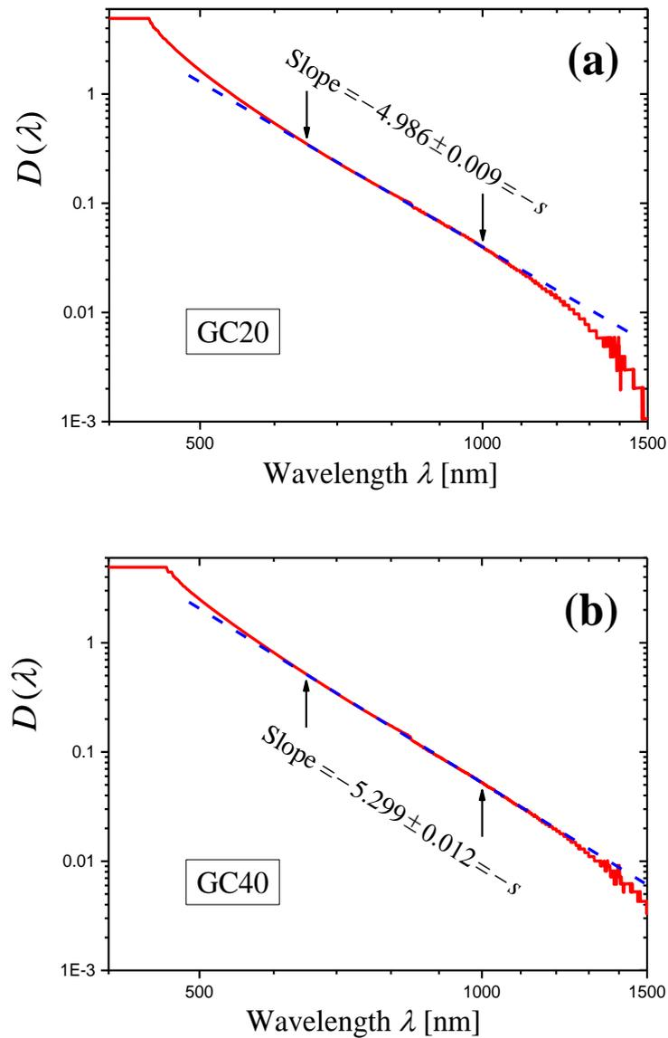
**Figure 10.** Log–log plots of the internal optical density  $D(\lambda)$  (red curves) for samples of the glass-ceramics GC20 (a) and GC40 (b). The samples have the same thickness  $h = 2.00$  mm. The portion of each curve limited by arrows is approximated by red dashed straight line using the least squares method, and the slope of the straight line is indicated in the figure.
