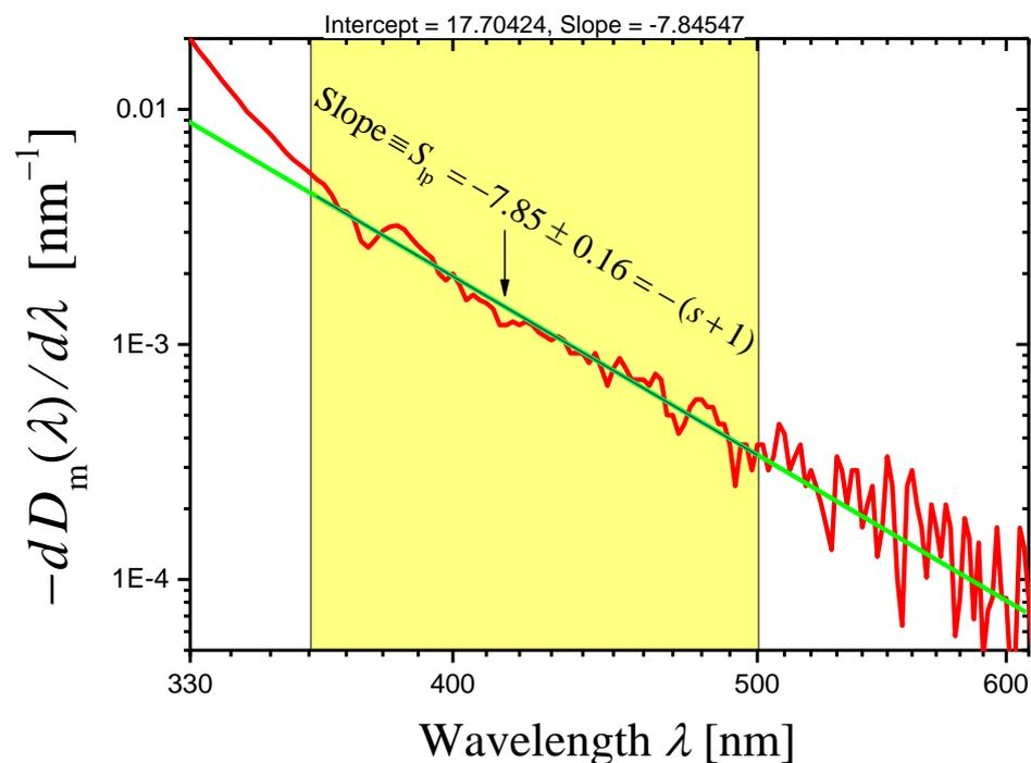
**Figure 1.** A log–log plot of the dependence of  $(-dD_m(\lambda)/d\lambda)$  on  $\lambda$  constructed for the measured optical density  $D_m(\lambda)$  of the glass G2 sample with the thickness  $h_2 = 10.00$  mm (red curve). The green straight line presents the linear least squares approximation of the curve in the spectral range of 360–500 nm.
