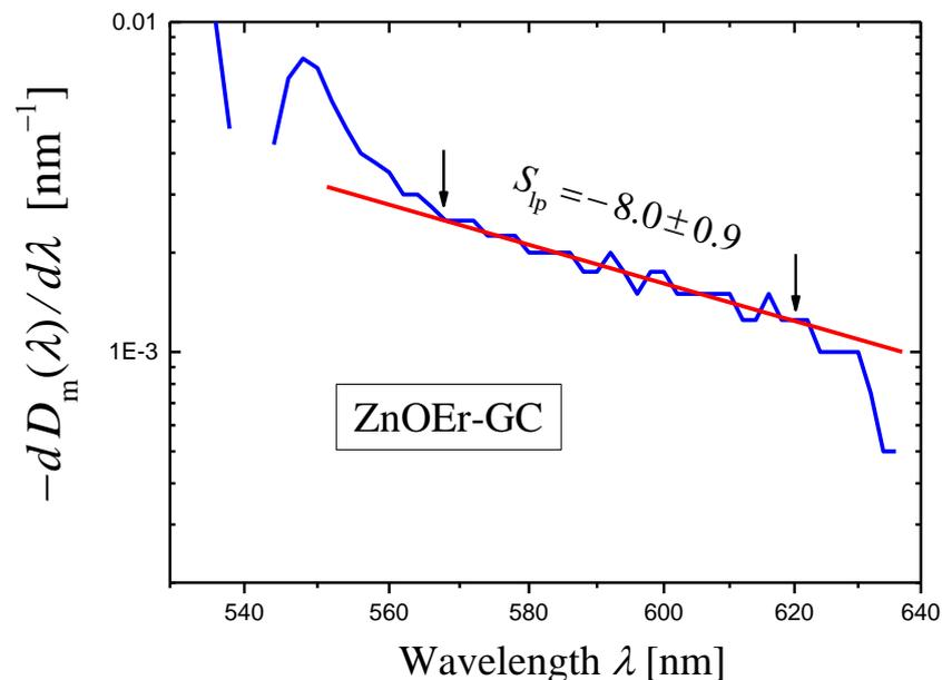
**Figure 7.** A log–log plot of the dependence of  $(-dD_{im}(\lambda)/d\lambda)$  on  $\lambda$  (blue curve) constructed for the measured optical densities  $D_m(\lambda)$  of sample of the glass-ceramic ZnOEr-GC. The sample thickness  $h = 1.06$  mm. The portion of the curve limited by arrows is approximated by a red straight line using the least squares method, and the slope  $S_{lp}$  of the straight line is indicated in the figure.
