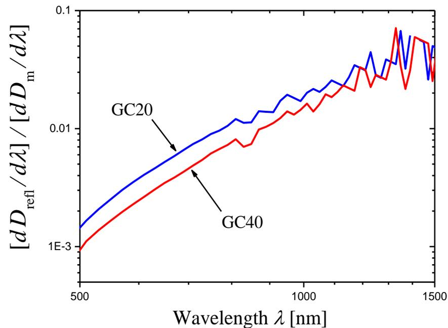
**Figure 14.** The ratio  $[dD_{\text{refl}}(\lambda)/d\lambda]/[dD_m(\lambda)/d\lambda]$  for the glass-ceramics GC20 and GC40. The wavelength step is  $\Delta\lambda = 20$  nm.
