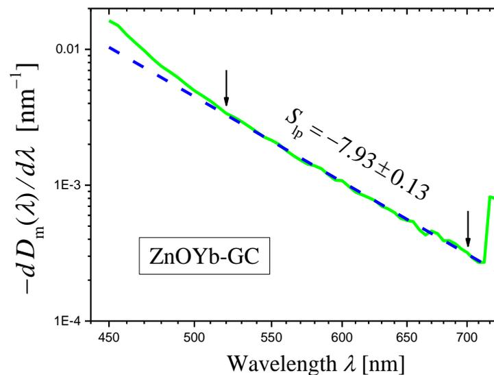
**Figure 12.** A log–log plot of the dependence of  $(-dD_{im}(\lambda)/d\lambda)$  on  $\lambda$  (green curve) constructed for the measured optical density  $D_m(\lambda)$  of sample of the glass-ceramic ZnOYb-GC with the thickness  $h = 3.02$  mm. The portion of the curve limited by arrows is approximated by blue dashed straight line using the least squares method, and the slope  $S_{lp}$  of the straight line is indicated in the figure. The wavelength step  $\Delta\lambda = 5$  nm was used.
