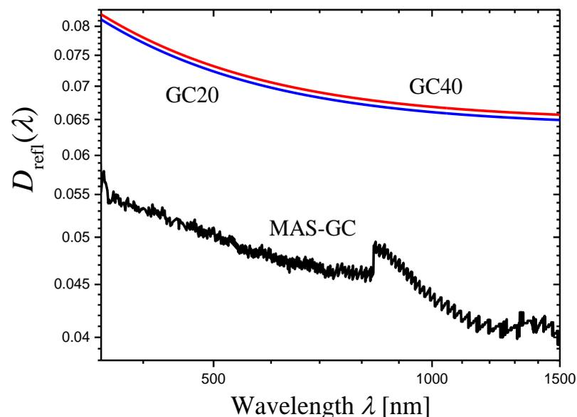
**Figure 13.** Optical densities of reflection losses,  $D_{\text{refl}}(\lambda)$ , calculated for the glass-ceramics GC20, GC40 and MAS-GC (log–log plots). For the glass-ceramics GC20 and GC40, Equation (6) and analytical expressions for refractive index  $n(\lambda)$  were used. In the case of the glass-ceramic MAS-GC, calculation was carried out by Equation (34) using the measured optical densities of two samples.
