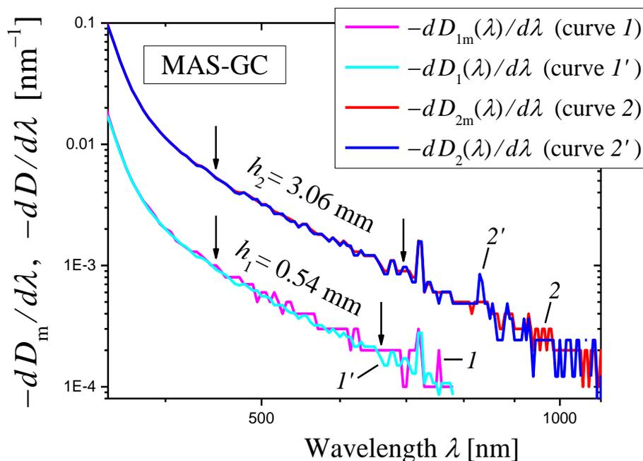
**Figure 15.** The plots of  $[\log_{10}(-dD_{im}(\lambda)/d\lambda)] - [\log_{10}(\lambda)]$  (curves 1 and 2) and  $[\log_{10}(-dD_i(\lambda)/d\lambda)] - [\log_{10}(\lambda)]$  (curves 1' and 2') for the thin ( $i = 1$ , curves 1 and 1') and thick ( $i = 2$ , curves 2 and 2') samples of MAS-GC (Section 2.2.4).
