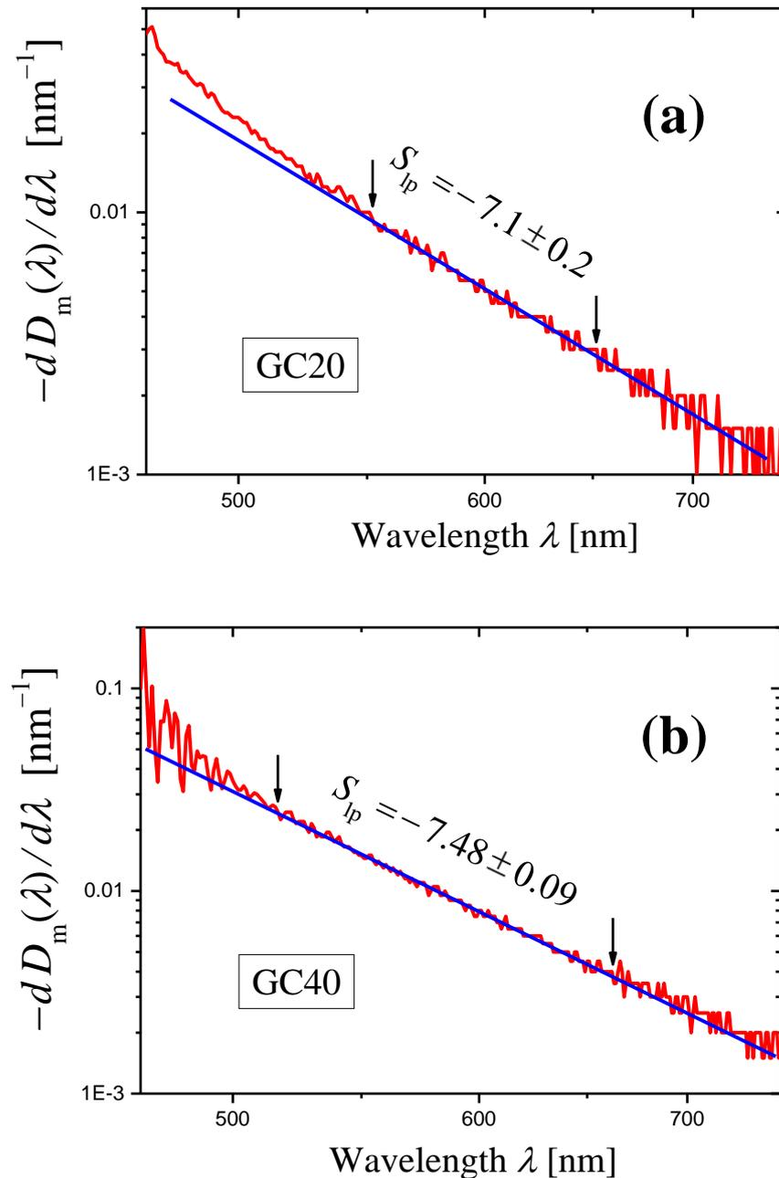
**Figure 6.** Log–log plots of the dependences of  $(-dD_{im}(\lambda)/d\lambda)$  on  $\lambda$  (red curves) constructed for the measured optical densities  $D_m(\lambda)$  of the samples of the glass-ceramics GC20 (a) and GC40 (b). The samples have the same thickness  $h = 2.00$  mm. The portion of each curve limited by arrows is approximated by blue straight line using the least squares method, and the slope  $S_{lp}$  of the straight line is indicated in the figure.
