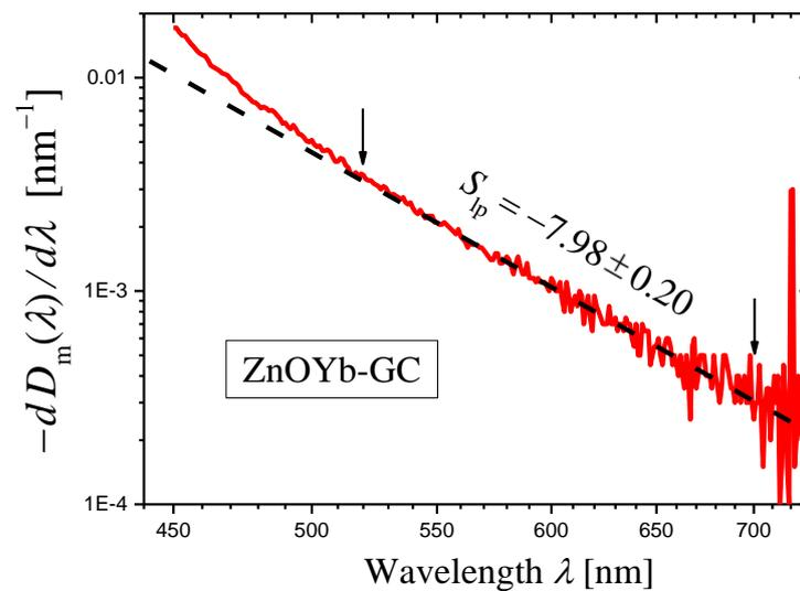
**Figure 9.** A log–log plot of the dependence of  $(-dD_{im}(\lambda)/d\lambda)$  on  $\lambda$  (red curve) constructed for the measured optical density  $D_m(\lambda)$  of sample of the glass-ceramic ZnOYb-GC with the thickness  $h = 3.02$  mm. The portion of the curve limited by arrows is approximated by a black dashed straight line using the least squares method, and the slope  $S_{ip}$  of the straight line is indicated in the figure.
