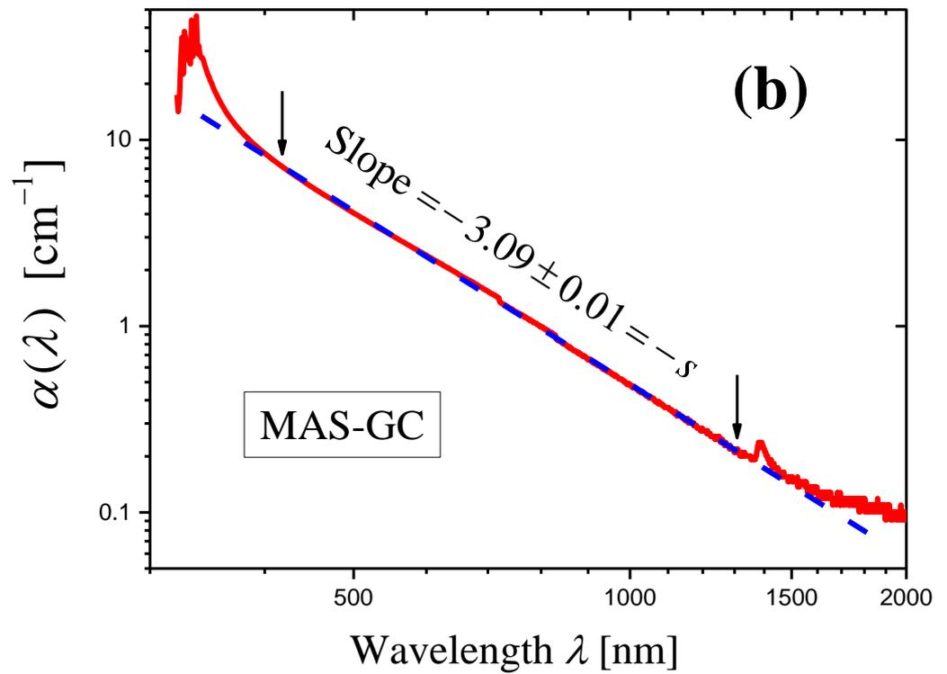
**Figure 4.** (a): Log–log plots of the measured optical densities for two samples of the MAS-GC with thicknesses indicated in the figure. (b): A log–log plot of wavelength dependence of the extinction coefficient  $\alpha(\lambda)$  determined by Equation (5) on the basis of the data presented in Figure 4a (the first method).
