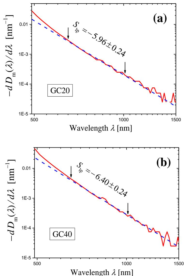
**Figure 11.** Log–log plots of the dependences of  $(-dD_{im}(\lambda)/d\lambda)$  on  $\lambda$  (red curves) constructed for the measured optical densities  $D_m(\lambda)$  of samples of the glass-ceramics GC20 (a) and GC40 (b). Notice that the spectral range is wider than in Figure 6 for the same glass-ceramics; the wavelength step  $\Delta\lambda = 20$  nm is greater than the step  $\Delta\lambda = 1$  nm used to draw the curves in Figure 6.
