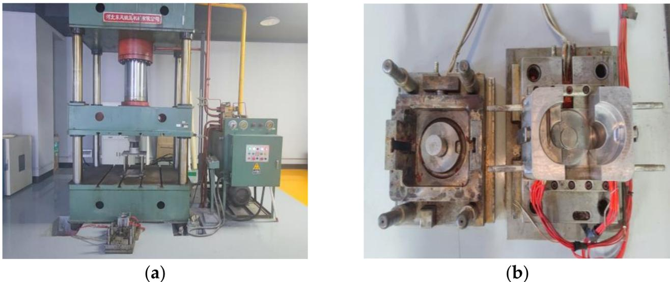
**Figure 2.** Experimental production equipment. (a) Hydraulic press. (b) Compression mold.
