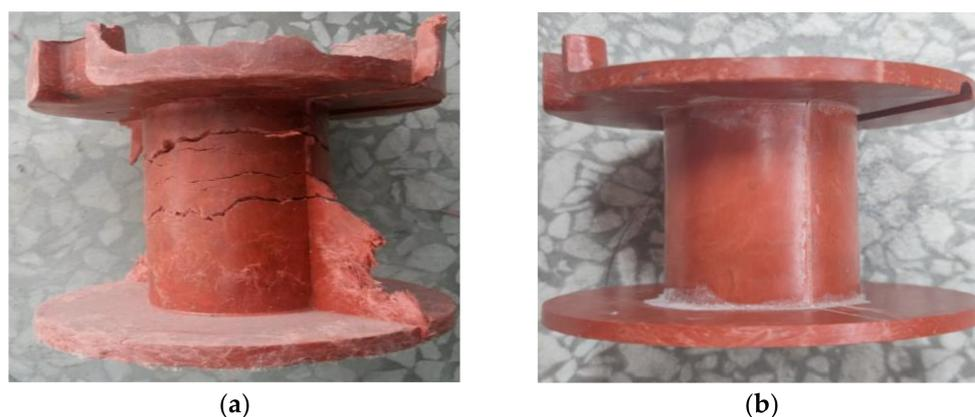
**Figure 3.** Compression-molded FRSR coil bobbin. (a) By process parameters recommended with the raw material supplier. (b) Process parameters optimized based thermal analysis tests.
