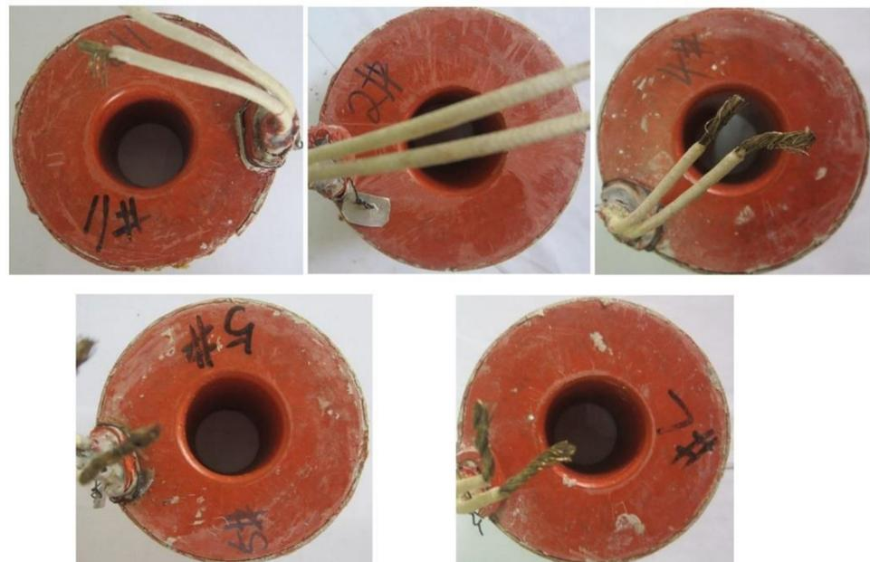
**Figure 12.** The coil assemblies after 7 days of heat exposure at 310 °C.
