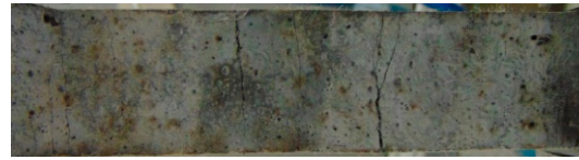
Figure 11. Multiple cracking pattern of tensile specimen for HDC.
