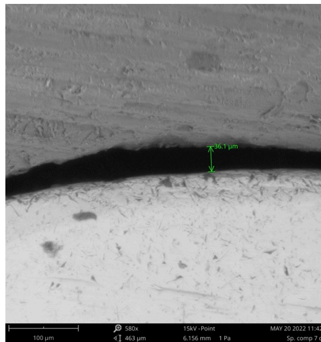
Figure 4. A 580× SEM image for evaluation of marginal gap at restoration-abutment interface.
