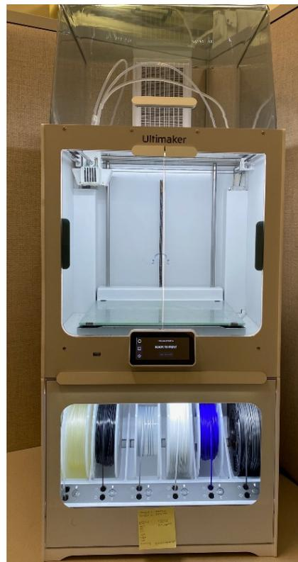
Figure 1. Image of Ultimaker© S5 printer.
