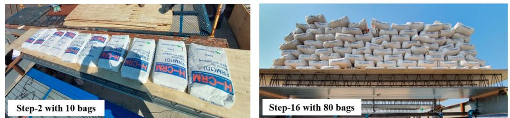
Figure 4. Photos at Step-2 with 10 load bags and Step-16 with 80 load bags.
