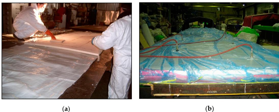
**Figure 1.** (a) Laying pre-pregs with polyurethane foam; (b) Using vacuum pump technology to consolidate panel layers (photo Mostostal Warszawa).
