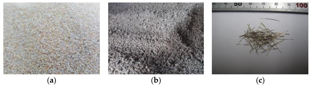
**Figure 2.** Fine aggregates and steel fiber used in this study: (a) Natural sand; (b) Recycled sand; (c) Steel fiber.
