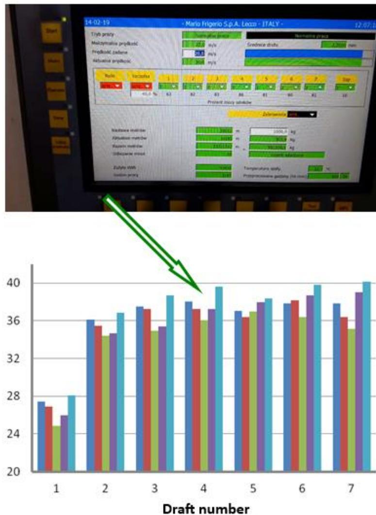
**Figure 7.** Control panel of the Mario Frigerio machine and percentage load of the engines P in respective drafts for the wires drawn with the angle  $\alpha = 3, 4, 5, 6$  and  $7^\circ$  and drawing speed of 20 m/s.
