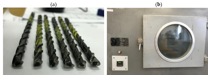
Figure 4. Preparation samples for mechanical tests; (a) One part of the samples prepared for the shear test, (b) The heating process of the samples at a stabilized temperature of 80\text{ }^{\circ}\text{C} .
