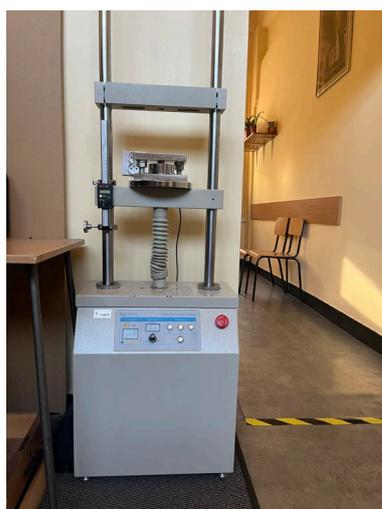
**Figure 3.** Sauter testing machine.
