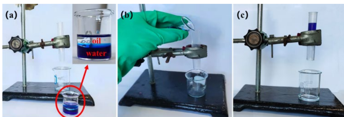
Figure 10. (a–c) Oil–water separation experiment of the SBS/C9-SiO 2 coatings.
