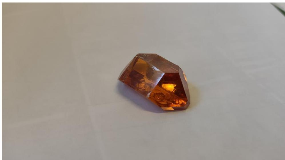
**Figure 2.** Bottom and side faces of the [110] BSO:Eu single crystal, as grown.
