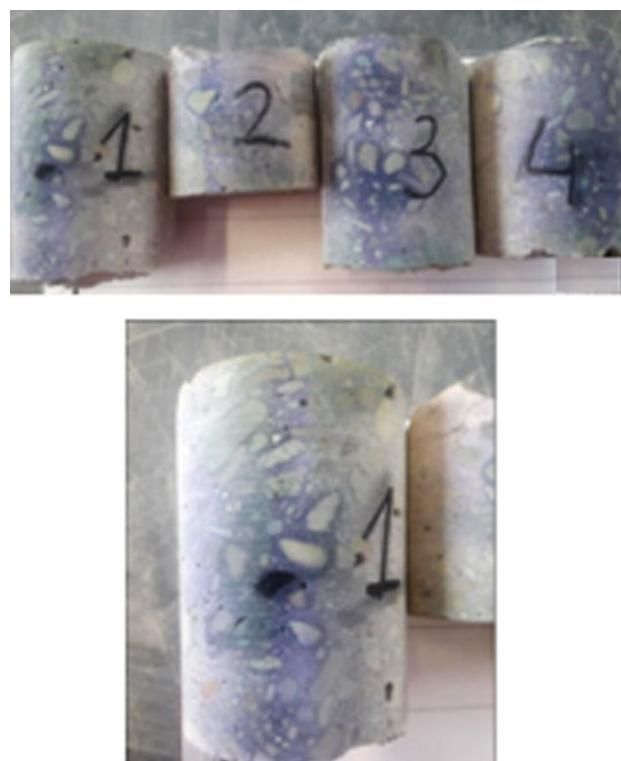
**Figure 9.** Test of the extension of concrete carbonation.
