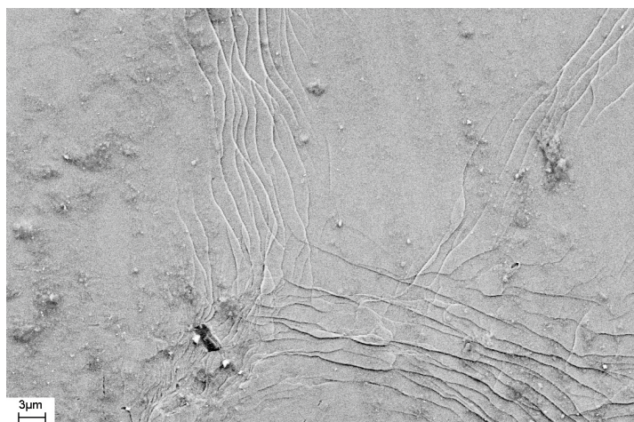
Figure 15. SEM image of the surface of the amorphous \text{Fe}_{77}\text{Si}_{13}\text{B}_{10} ribbon deformed by rolling (one rolling pass).
