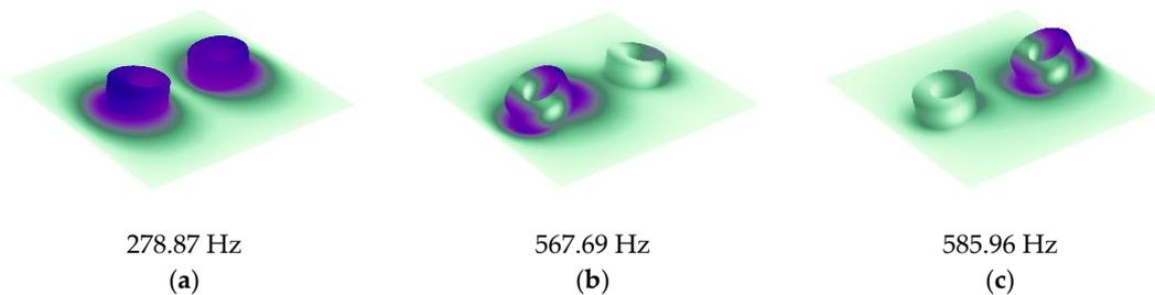
**Figure 7.** Eigenmodes of the double-mass-loaded membrane: (a) 278.87 Hz, (b) 567.69 Hz, and (c) 585.96 Hz.
