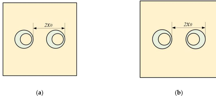
**Figure 5.** Definitions for the configuration of the MAM loaded with two masses: (a) asymmetric arrangement and (b) symmetric arrangement.
