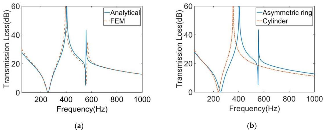
**Figure 3.** (a) Comparison of the analytical and numerical results for the STL curve of the MAM with an asymmetric ring. (b) Comparison of the MAMs with an asymmetric ring and a cylinder for the STL curve.
