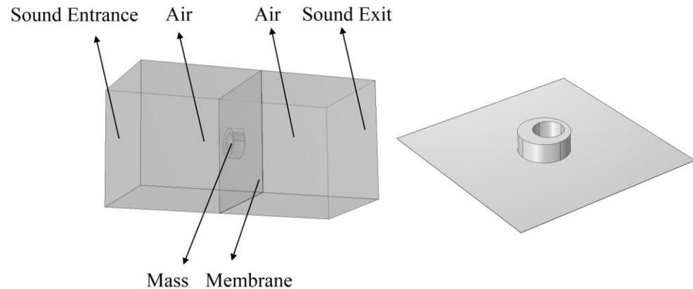
**Figure 2.** The 3D finite element model for the verification of the analytical model.
