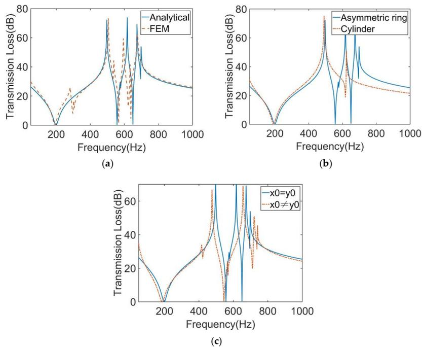
**Figure 9.** (a) Comparison of the analytical and numerical results for the STL curve of the MAM with four asymmetric rings. (b) Comparison of the MAMs with four asymmetric rings and four cylinders for the STL curve. (c) Comparison of the MAMs with mass positions  $x_0 = y_0$  and  $x_0 \neq y_0$  for the STL curve.
