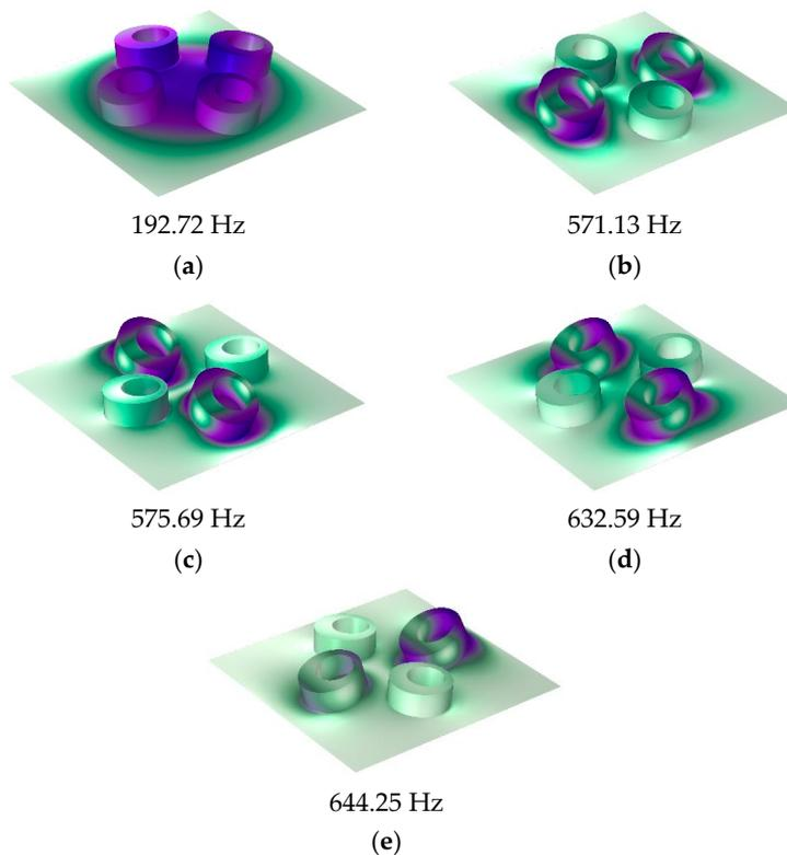
**Figure 10.** Eigenmodes of the four-mass-loaded membrane: (a) 192.72 Hz, (b) 571.13 Hz, (c) 575.69 Hz, (d) 632.59 Hz, and (e) 644.25 Hz.
