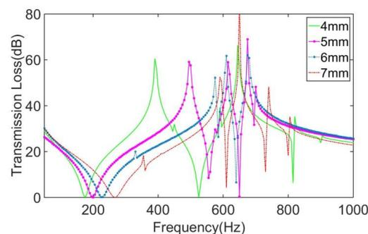
**Figure 12.** Comparison of the MAMs with different mass positions.
