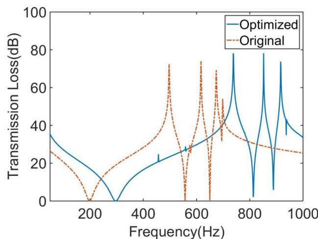
Figure 17. Comparison of the original and optimized MAMs for the STL curve.
