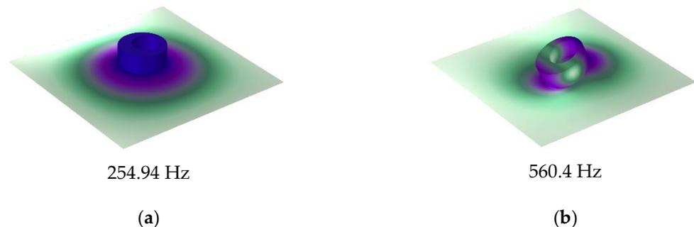
**Figure 4.** Eigenmodes of the single-mass-loaded membrane: (a) 254.94 Hz and (b) 560.4 Hz.
