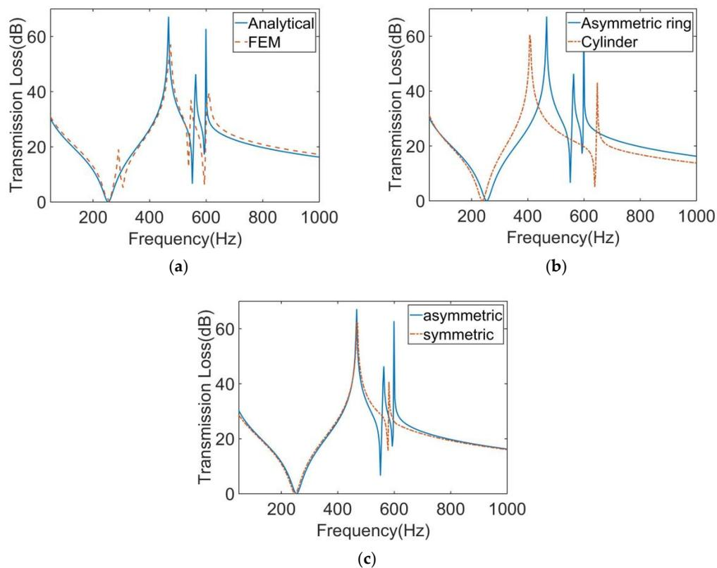
**Figure 6.** (a) Comparison of the analytical and numerical results for the STL curve of the MAM with two asymmetric rings. (b) Comparison of the MAMs with two asymmetric rings and two cylinders for the STL curve. (c) Comparison of the MAMs with two asymmetric rings, asymmetrically and symmetrically arranged.
