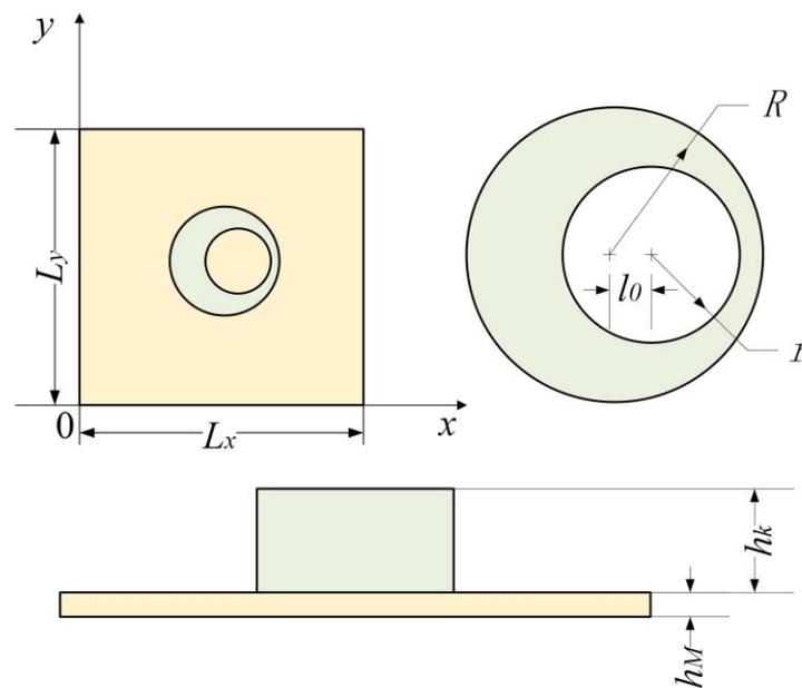
**Figure 1.** Definitions for the configuration of the MAM loaded with an asymmetric mass.
