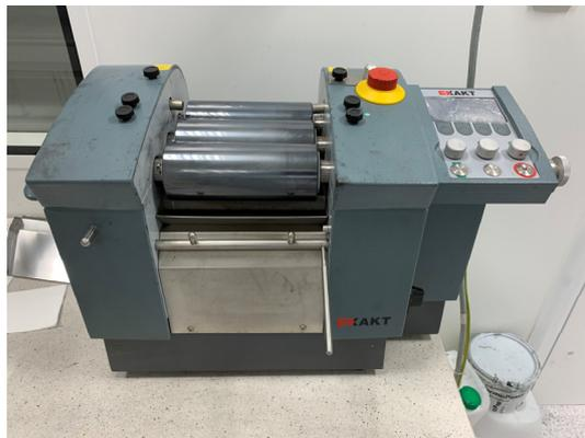
**Figure 1.** Three-roll mill EXAKT model 80E.
